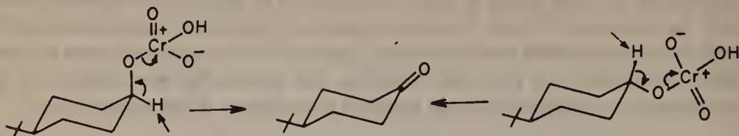
Figure 12.32 Mechanism of chromic acid oxidation
