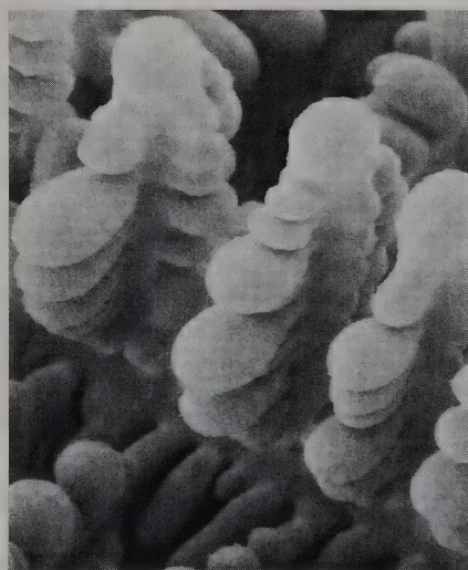
Directionally solidified iron dendrites from an iron-copper alloy after dissolving away the copper (magnification x 2600)
