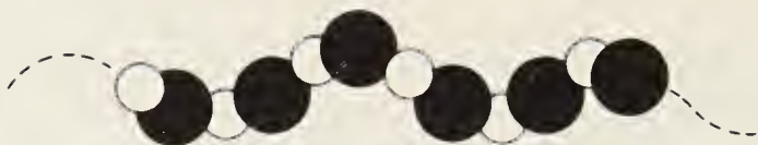
Figure 31. Helical lattice of cinnabar. Mercury atoms (black) alternate with sulfur atoms (white).
