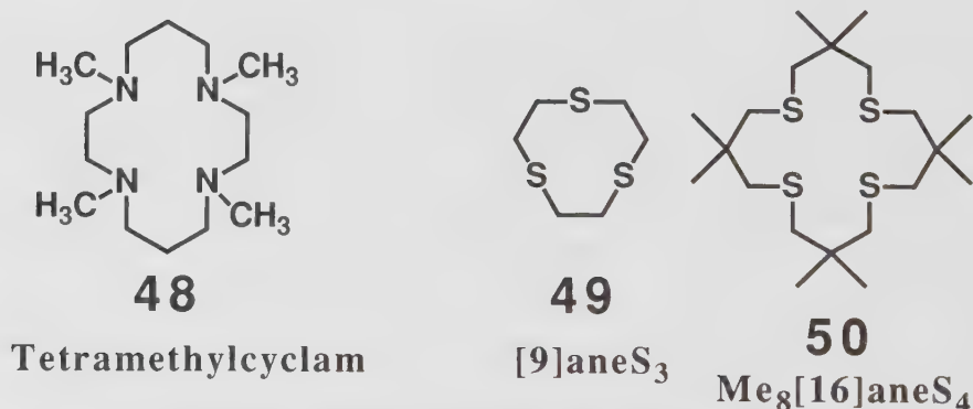
Figure 6.17. Macrocyclic ligands to stabilize lower oxidation states of metal ions.
