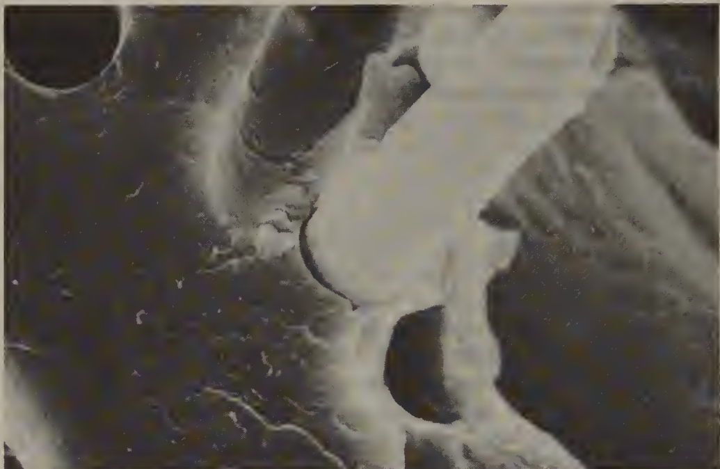
FIGURE 7.5.1. Micrograph of a carbon fiber-reinforced composite fracture surface. [Reprinted with permission from Materials Science and Engineering for the 1990s: Maintaining Competitiveness in the Age of Materials , National Academy Press, Washington, DC, 1989. Copyright 1989 E. I. Du Pont de Nemours & Co., Inc.]
