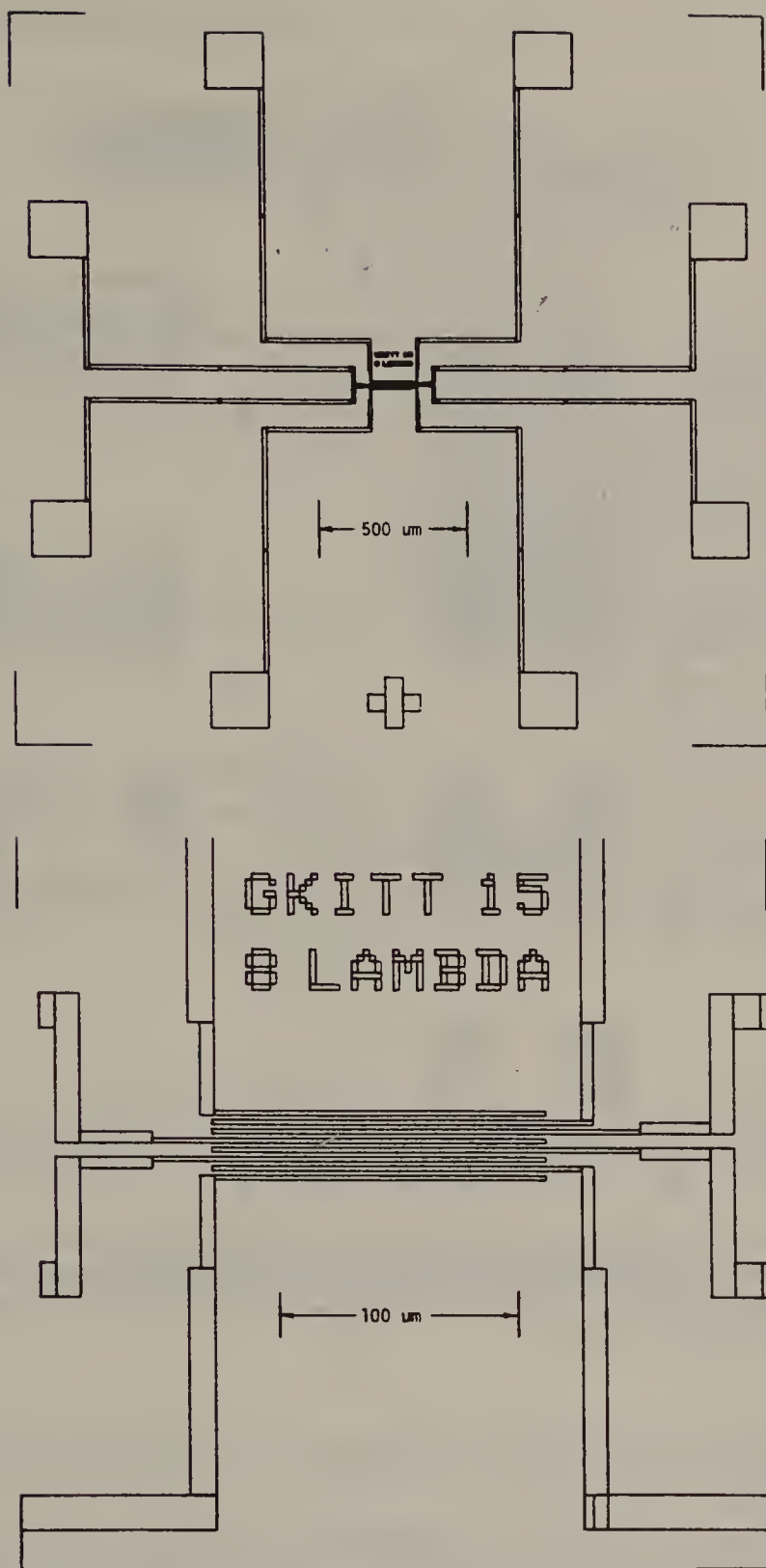
FIGURE 4.8.7. Layout of typical microelectrode array at two different size scales, showing (above) the contact pads and (below) the details of the electrode array structure. Typical arrays comprise electrodes of Pt or Au formed on oxidized Si wafers. [Reprinted with permission from G. P. Kittlesen, H. S. White and M. S. Wrighton, J. Am. Chem. Soc. , 106 , 7389 (1984). Copyright 1984 American Chemical Society.]
