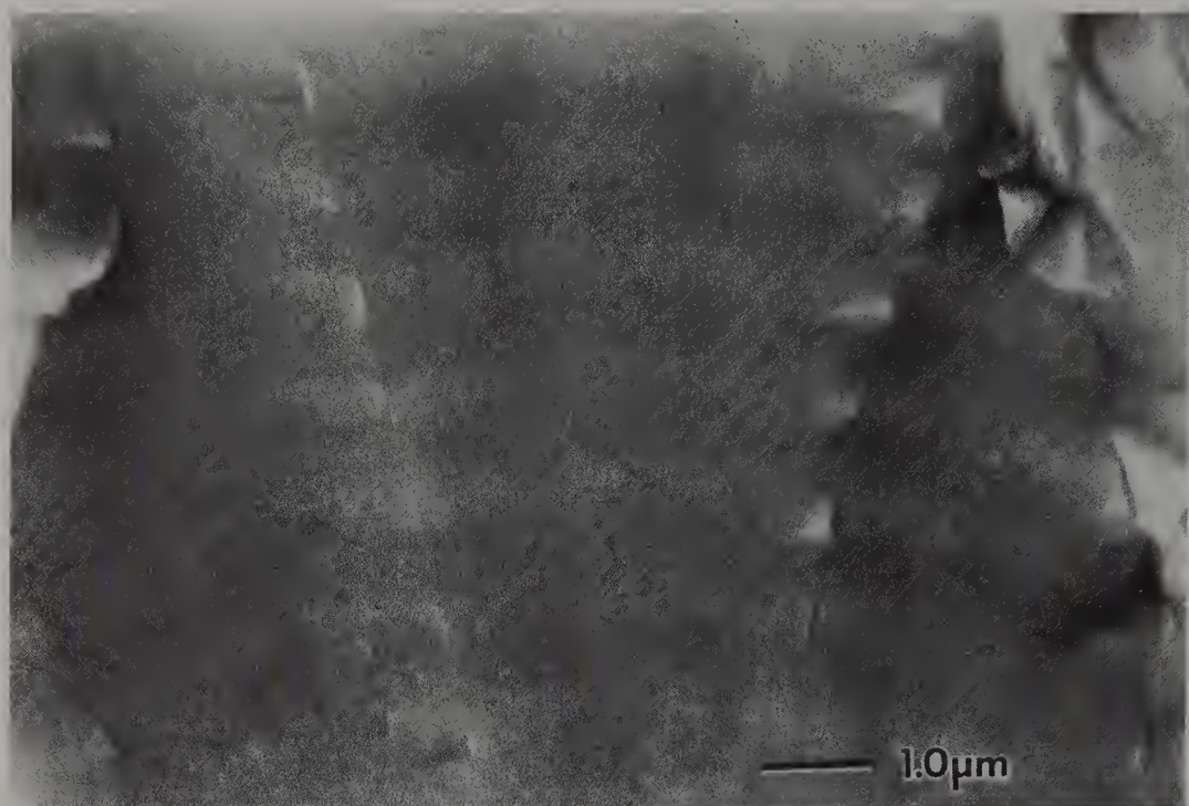
Figure 5. Scanning electron micrograph of a modulated \text{Tl}_a\text{Pb}_b\text{O}_c/\text{Tl}_d\text{Pb}_e\text{O}_f film. A cross-sectional view of a fractured film is shown. The film was deposited by cycling between 0.05 \text{ mA/cm}^2 and 5 \text{ mA/cm}^2 in a solution of 0.005 \text{ M TiNO}_3 and 0.1 \text{ M Pb(NO}_3)_2 in 5 \text{ M NaOH} . Layer thicknesses are intentionally quite thick ( \sim 0.5 \mu ) so that SEM imaging is possible.
