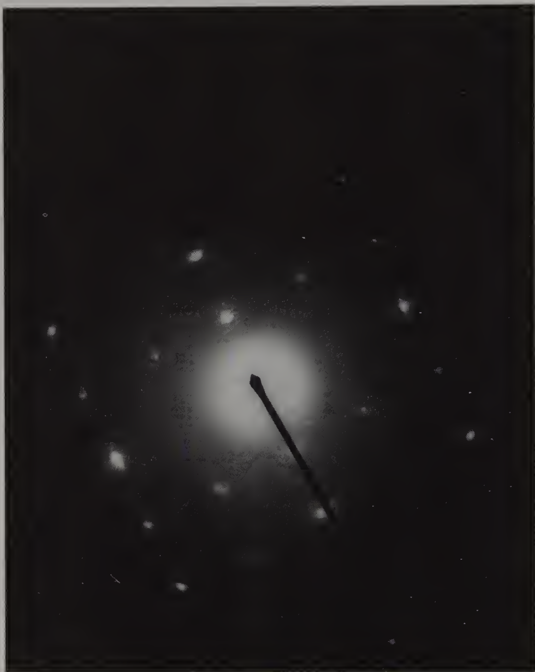
Figure 6. Selected area diffraction pattern of crystallites of polyfuran/FeOCl (II) with the beam perpendicular to the (101) plane showing the crystalline nature of the material.
