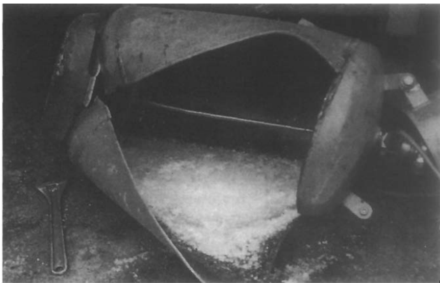
Figure 4-3. The result of pressurizing a cylinder to “two divisions” on a scale graduated in kg/cm 2 instead of psi. ( Photo courtesy of the Institution of Chemical Engineers. )
