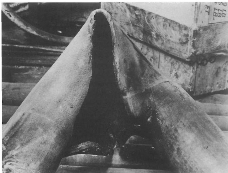
Figure 9-12. An old pipe was reused and failed by creep.
