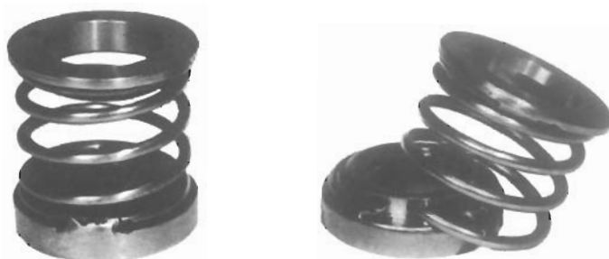
Figure 10-7. End caps welded to spring. Failure occurred at weld.
