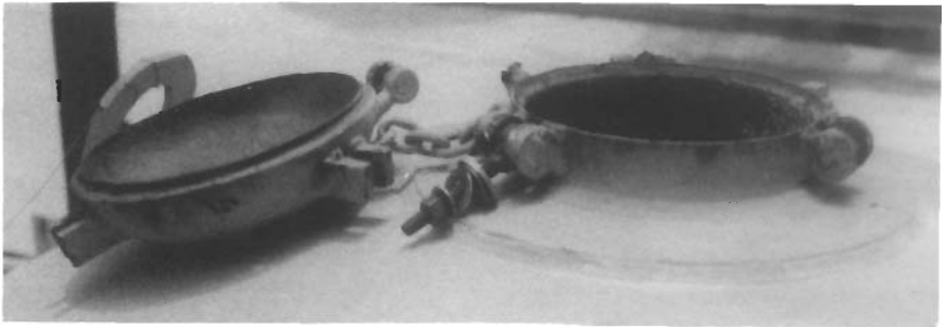
Figure 1-18. Instead of replacing the eye-bolts, new studs were welded in place of the threaded portions. They were made brittle by the heat and failed in use. Fortunately the chain prevented the lid from going into orbit.
