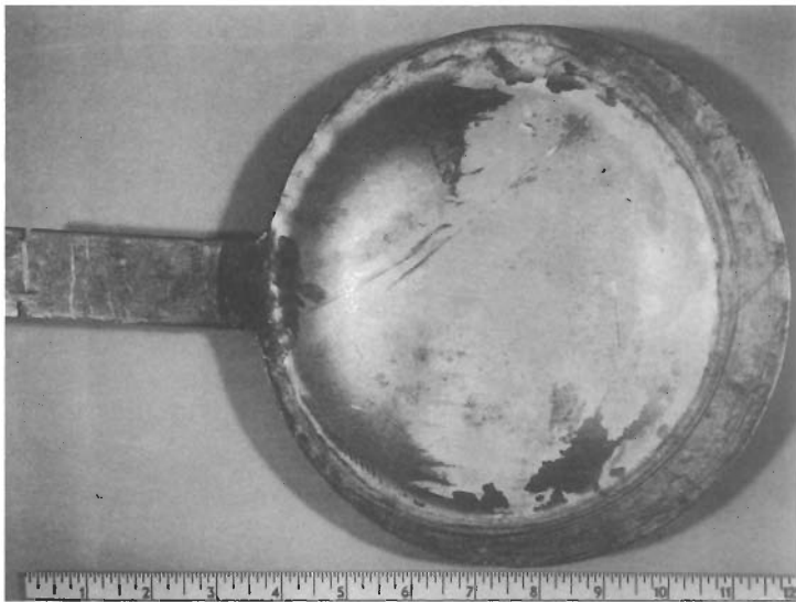
Figure 1-6. A slip-plate bowed by a gauge pressure of 470 psi (32 bar).
