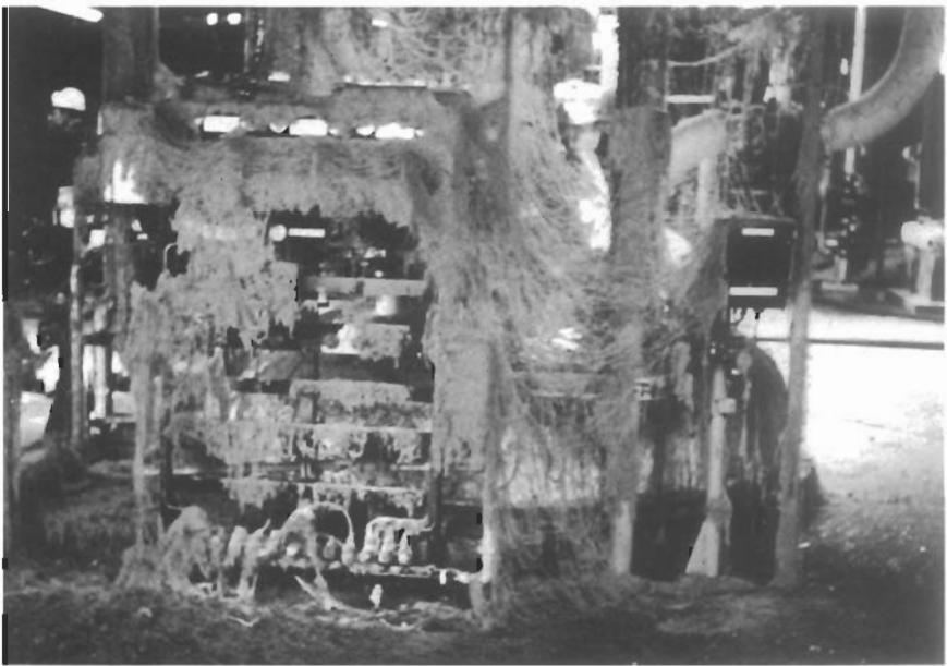
Figure 3-1b. Because a rupture disc was fitted to the wrong side of a vacuum support, the flanges leaked, covering the reactor with "candy."
