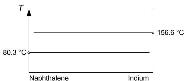
Figure 13.2. Empty phase diagram obtained with inert substances. Any mixture shows both melting points and does not exhibit any interactions. The crucible and sample in thermal analysis should behave in this way.
