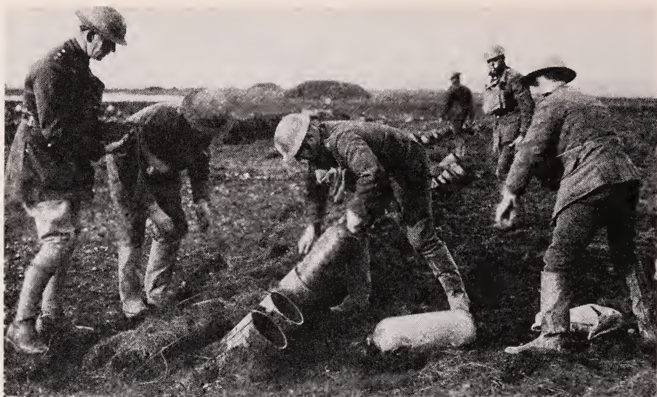
The British chemical weapon that the Germans feared most. Livens Projectors, fired in batteries of 25 at a time; each sent a drum of 30 pounds of liquid phosgene hurtling into the enemy's lines. ( Imperial War Museum )
