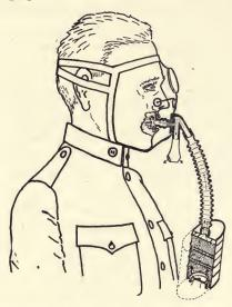
Fig. 53.—Diagrammatic Sketch of Box Respirator Type Mask.
