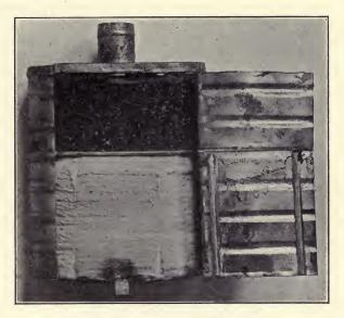
Fig. 104.—Crepe Paper Doughnut Filter Canister.
