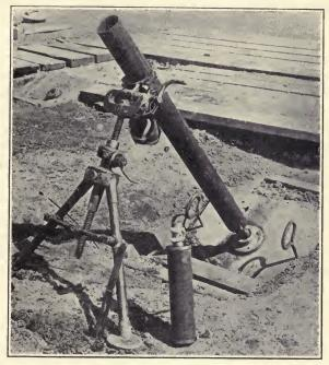
Fig. 3.—Stokes' Mortar.
