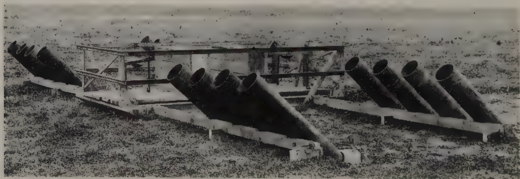
Tank sledge deployed and extended, with sixteen projectors resting on slots in the extended sledge ready for firing. (Courtesy of Liddle Collection, Leeds)
