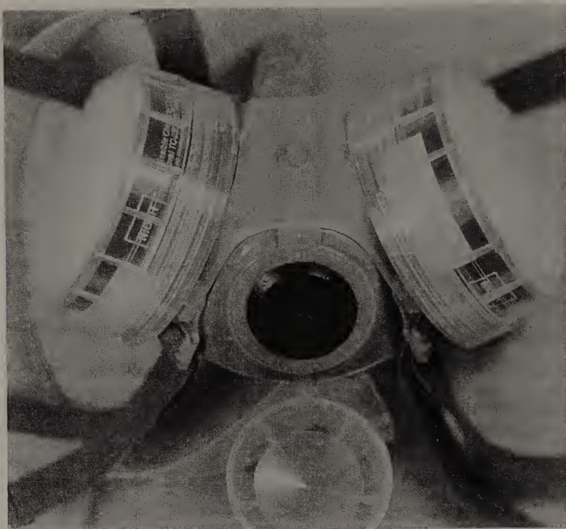
FIGURE 18-9 A close-up of the civilian painter's mask. The two large white objects are the filter element showing a fabric dust filter. Air is drawn in during breathing through the two filter elements directly to the nose and mouth. Unlike the military protective masks, this type of mask with no eyelenses does not require passage of the intake air across the lenses for defogging as there are no eyelenses. The smaller, black circular object at the bottom of the mask is the exhaust valve assembly (the plastic cover opened).
