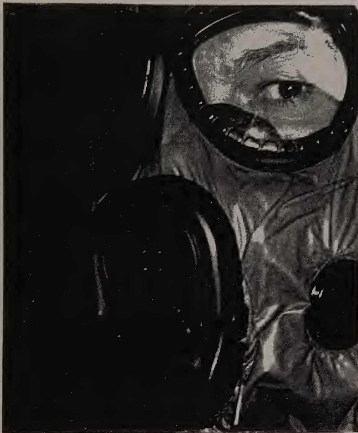
FIGURE 18-5 The M17A1 Protective Mask as worn by a real soldier. The black circular object in front of the mask at the nose of the wearer houses the voicemitter and the exhaust valve is below the voicemitter under the black rubber cover flap at the bottom. The long object just below the voicemitter is a drinking tube which attaches to the canteen under combat conditions. The smaller black circular object to the right of the picture under the eye piece is the intake valve assembly cover. Air enters through it, passes over and through the toxic agent filter element located within each cheek pouch of the mask body and the air passes into the interior of the mask by flowing over the transparent eyelens. This airflow arrangement is intended to act as a defogger to permit clear vision through the eyelenses. [Courtesy U.S. Army]
