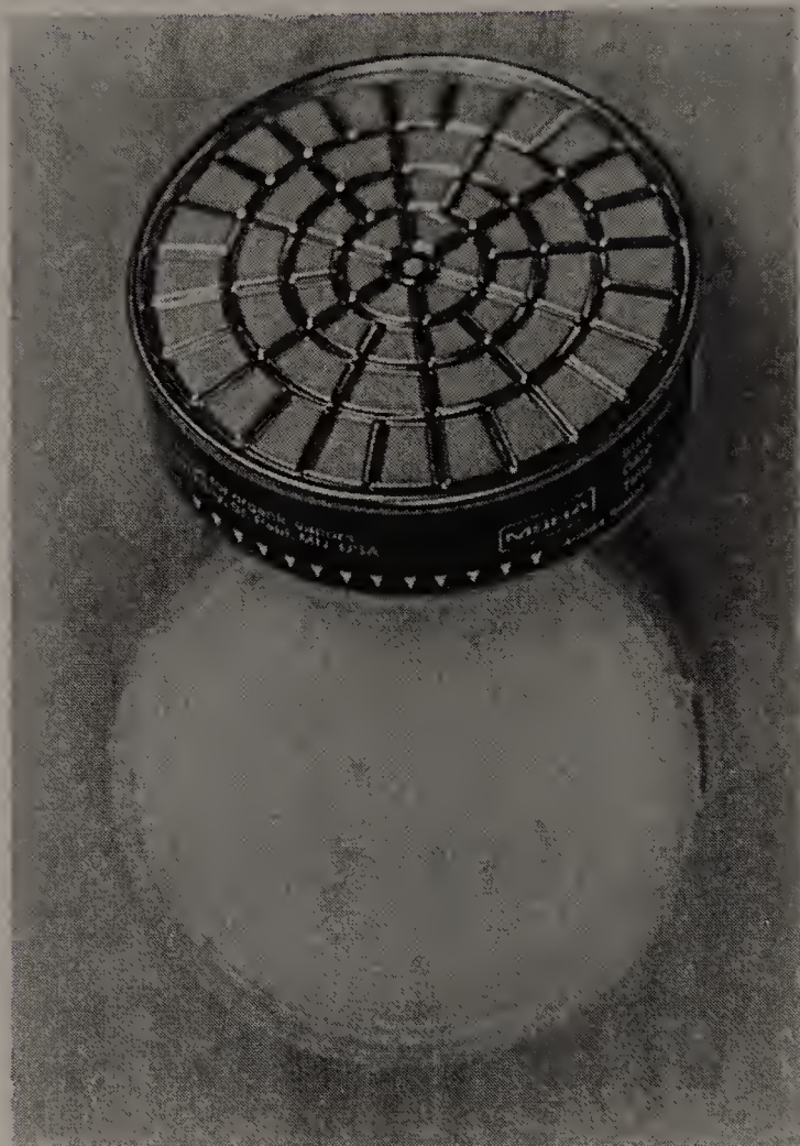
FIGURE 18-11 A filter element unit showing the thin fabric (white) cover over the activated charcoal component. The white circular object is the cover assembly which screws onto the mask filter element housing, holding the filter element securely in place.
