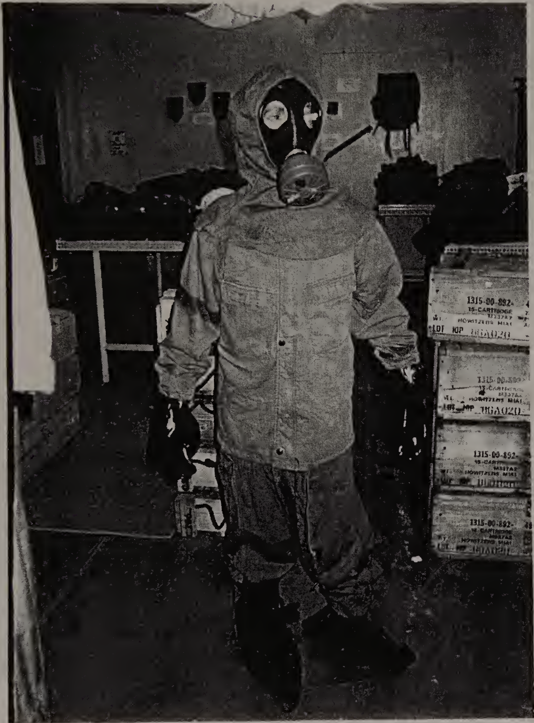
FIGURE 18-1 Protective Gear : A mannequin dressed out in protective mask, impermeable overgarment, rubberized gloves and hood with rubberized boots. Note that the hood covers over the shoulders. Straps are provided for tying under the armpits. Also, the trousers seal around and below the top of the rubberized over-boots. [Courtesy Dixie Surplus, Lafayette, LA]
