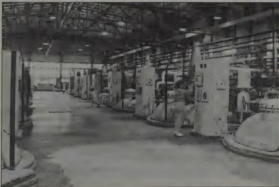
Photograph of SNOB's Building 221 interior with a row of 20,000 liter fermenters. (Photographer: Andrew C. Weber.)
