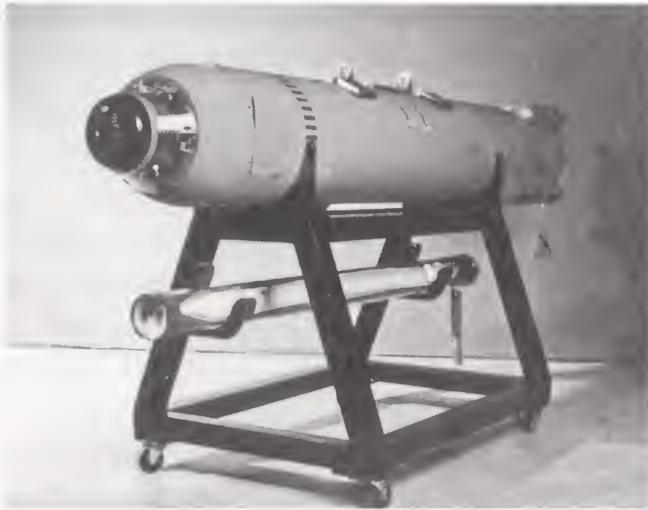
A mock-up of the Bigeye bomb, an aircraft-delivered binary weapon that was designed to produce VX by combining two relatively non-toxic precursors (QL and powdered sulfur). The bomb would glide to earth while spraying nerve agent over the target. Because of chronic technical problems, the Bigeye bomb was never produced.
