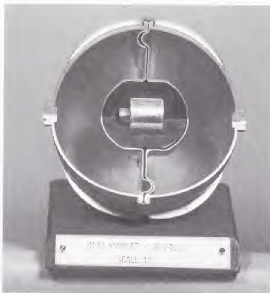
Cutaway of an M139 Sarin bomblet shows internal cavities that were filled with liquid Sarin. At its center are a fuse and an explosive burster that detonated on impact, generating a fine mist of nerve agent.
