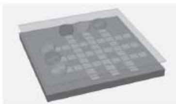
Figure 2. Schematic of EWOD-based micro-fluid chip and actual 5- \mu L droplet on electrode array.
