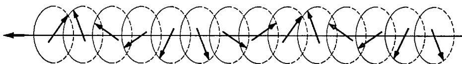
Fig. 6. Helical arrangement of dipoles along transverse axis
