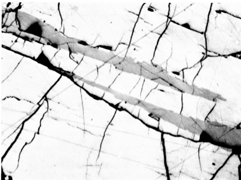
Fig. 12. Coarse daubreelite lamellae ( \text{FeCr}_2\text{S}_4 ) and a finely dispersed second generation exsolved from troilite ( \text{FeS} ) parallel to (0001); cleavage and cracks of shrinkage are visible. Mundrabilla meteorite, oil immersion, \times 400
