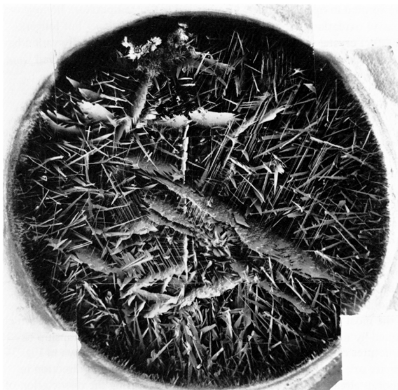
Fig. 52. Typical growth of alumina whiskers in an alumina crucible
