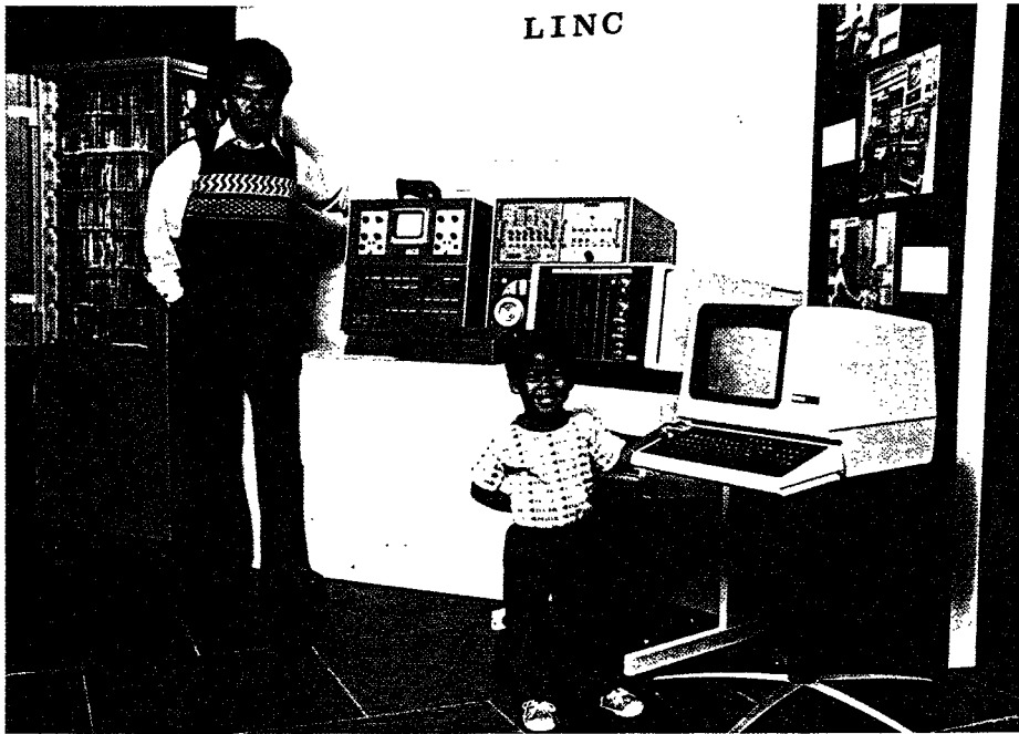
Fig. 4. Two generations of laboratory computers: on the left, the LINC from 1962 and on the right the MINC from 1978. Although the MINC is about a quarter of the size of the LINC it contains sixteen times as much memory, as well as a far more powerful processor. (Reproduced by courtesy of Digital Equipment Co.)
