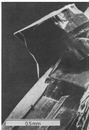
Fig. 10. Intergrowth of \alpha -TeI (compact crystal) and \beta -TeI (fibrous crystal) 18) ; SEM-photograph
