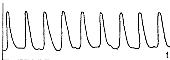
Fig. III.6. Oscillations of colored solution of Belousov reaction (After Zhabotinskii (1964-1))
