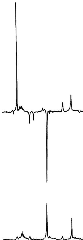
Fig. 25. Time resolved CIDNP spectrum observed upon photo-induced electron transfer oxidation of hexamethyl-(Dewar)-benzene (0.02 M) by chloranil (0.02 M). The top spectrum was observed 5 \mu s after excitation with the frequency-tripled output (355 nm) of a Nd/YAG laser. The bottom spectrum was recorded in the dark
