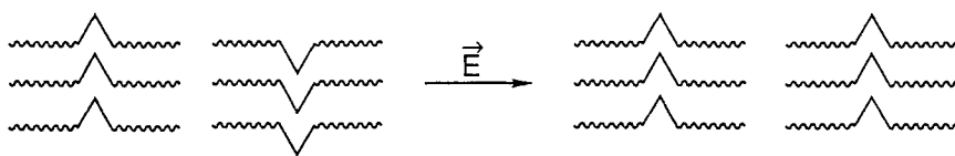
Fig. 19. Antiferroelectric to ferroelectric transition in a columnar mesophase made of molecules with a cone-shaped core
