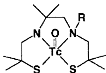
Fig. 8. Example of ^{99m}\text{TcO} -DADT bifunctional chelating agents R = sidechain for attachment to biomolecule
