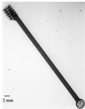
Fig. 19. Sieve with integrated cables (length 21 mm) and connection pads (light micrograph)
