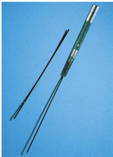
Fig. 2. Photograph of a flexible polyimide-based in vivo sensor for glucose, lactate and pH measurements
