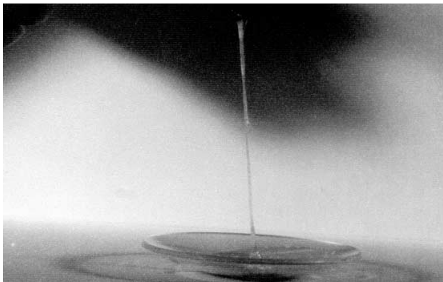
Fig. 2. A typical polythionylphosphazene elastomer (27 c)
