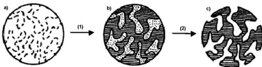
Scheme 1a–c Synthesis and structure of macroporous resins. a Polymer network forming; b porogen phase acts as pore template; c dry macroporous resin with large interconnected pores. (1) Porogen and network start to phase separate; (2) porogen phase removed to yield pores (hatched area=crosslinked polymer, dots=porogen phase)
