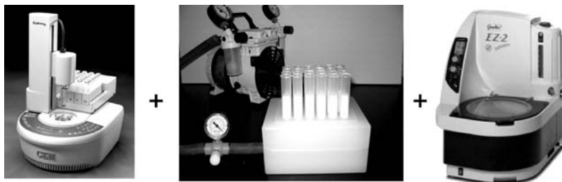
Fig. 2 A microwave-assisted fluorous synthesis system, microwave reactor ( left ), plate-to-plate SPE ( middle ), and a plate centrifuge unit ( right )
