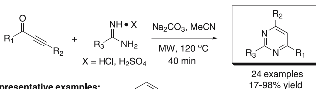
Scheme 45 A single-step synthesis of pyrimidines
