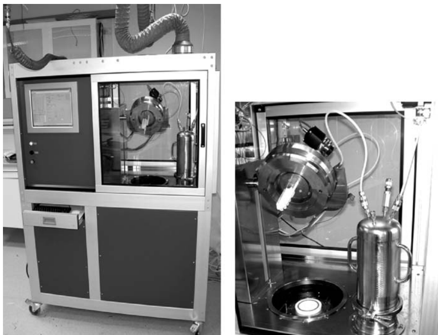
Fig. 9 Biotage Emrys Advancer Scale-Up and its multifunctional chamber head ( right )
