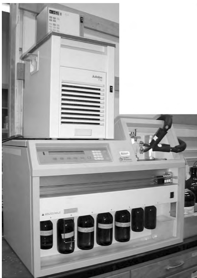
Fig. 3 Modified peptide synthesizer
