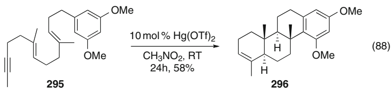
Scheme 52 Domino hydroarylation/cycloisomerization reactions of dienynes
