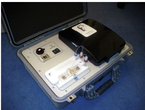
Fig. 11 Top: Integrated smart RNA hybridization sensor composed of sensing unit, preconcentration unit, and dehybridization unit. Bottom: A functioning prototype measuring 25 \times 10 \times 40 cm is shown in which a glass chip (like that shown in Fig. 10 but containing the multitarget design) is seen at the top of the instrumentation. A handheld prototype is expected in a year
