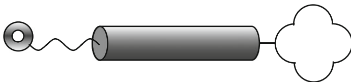
Fig. 1 Rod-like mesogen with terminal crown ether
