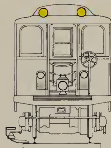
FORWARD END OF LIGHT TRAIN (ONE BOX LAMP ONLY ON RAPID TRANSIT DIVISION)
