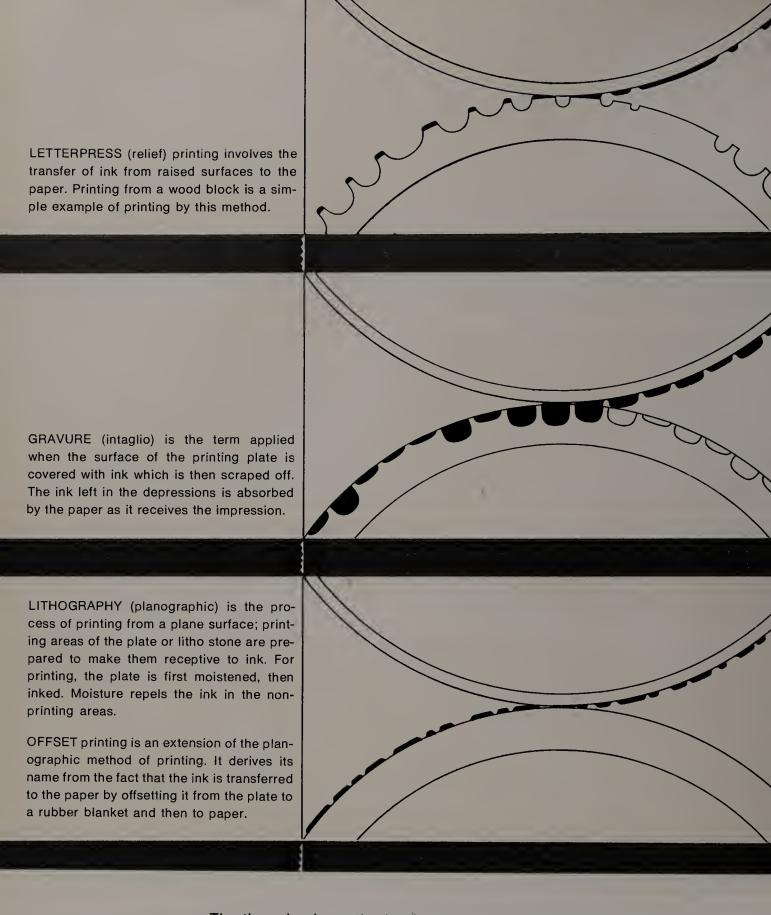
The three basic methods of printing are diagrammed in the columns above. While confusing trade names are sometimes applied to one method or another, essentially the methods are spoken of as letterpress, gravure and offset.
