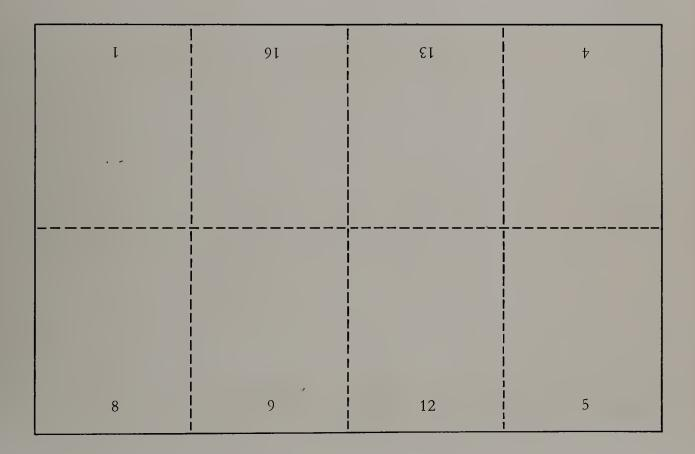
the extra colors are often printed on one side of the sheet only; the position of the colors (imposition) is computed and the mechanicals are prepared accordingly. The diagram above shows a possible imposition of pages to take advantage of a second color on 8 pages of a 16-page form. By experimenting the designer can position a second color to his best advantage. The photograph at left shows how paper can be folded to find the position of the color.
