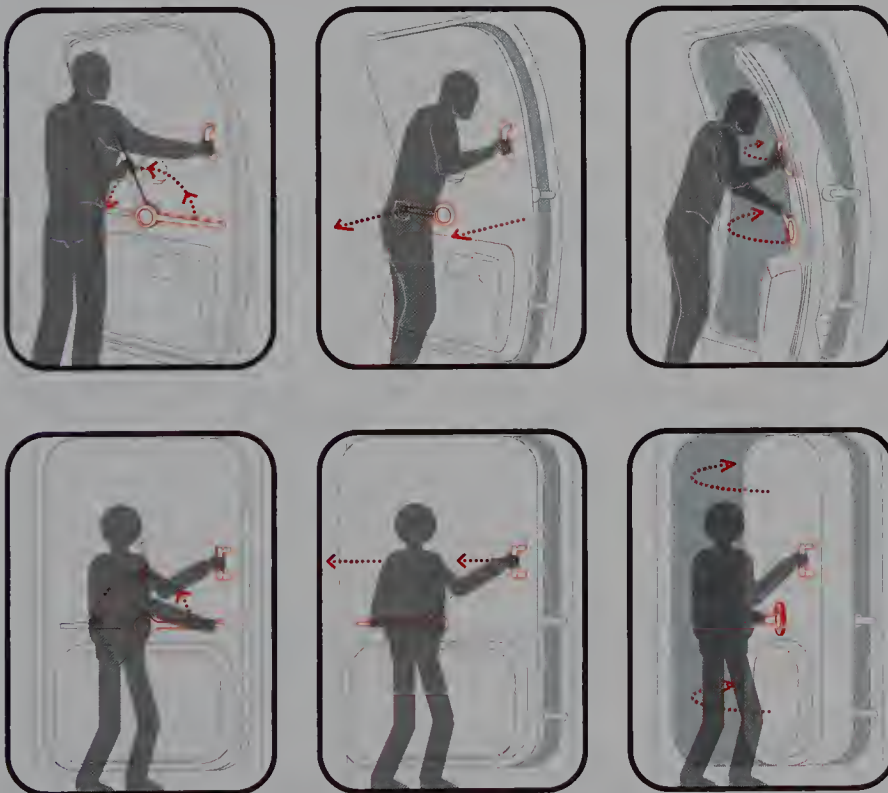
Figure 7.2 Two step-by-step explanations of how to open an airplane door in case of an emergency.
