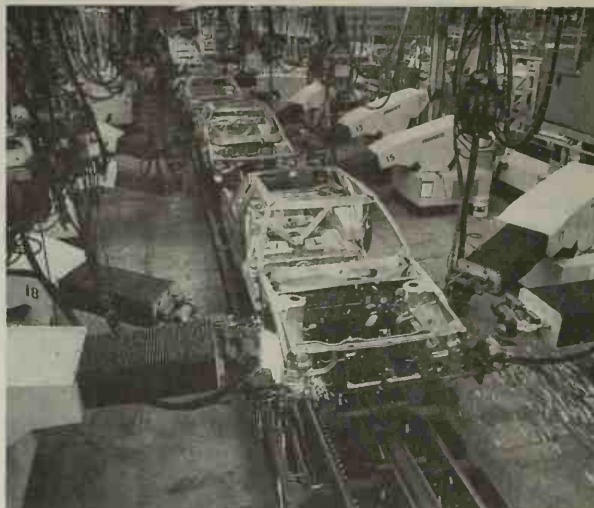
ASSEMBLY LINE. Robots welding at the Chrysler Corporation St. Louis Assembly Complex in Fenton, Missouri.
