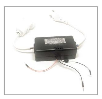
These components allow us to easily control devices powered by the mains electricity from an Arduino board, as you can just plug it into the mains electricity and then plug your device into it as well.
