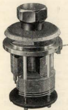
Fig. 6.11—Dual-range variable air capacitor (Type C853A) with screening cover removed; maximum inaccuracy 0.03 per cent. (H. W. Sullivan Ltd.)
