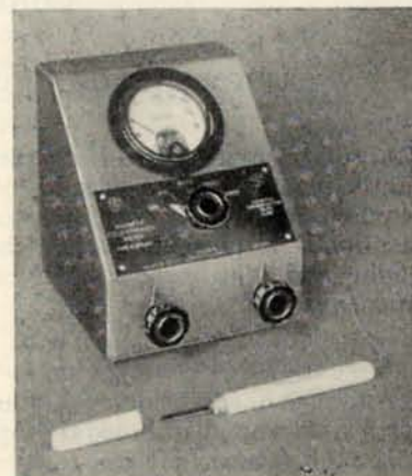
Fig. 10.13—B.T.-H. direct-reading flux-meter, employing the Hall effect in germanium. The point of the probe is held in the magnetic field to be measured
