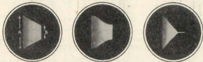
Fig. 11.18—C.r.t. traces from which the purity and depth of modulation can be determined
