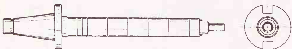
Figure 14-2 Typical milling-machine arbor, Style A. Note the pilot, which turns in the bearing in the arbor support. (Courtesy Cincinnati Milacron Company.)
