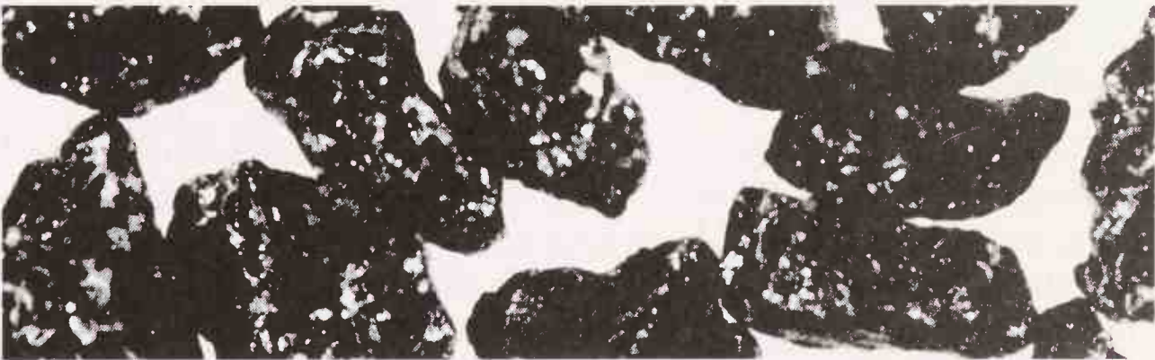
Figure 4-5 Regular aluminum oxide. This is a tough abrasive, well suited for general-purpose grinding, nonskid surfaces, barrel finishing, lapping, pressure blasting, and polishing. (Courtesy American Abrasive Company.)
