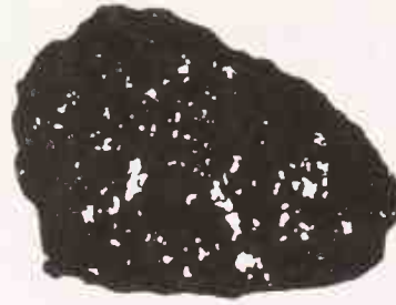
(C) Regular aluminum oxide abrasive.
