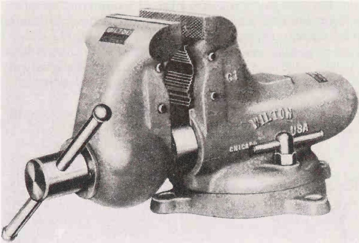
Figure 1-2 Combination vise. The inner teeth are for holding either pipe or round stock. (Courtesy Wilton Tool Mfg. Co.)
