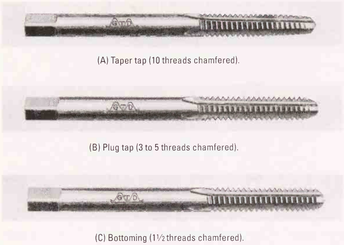
Figure 11-5 Set of three hand taps used in succession for tapping a blind hole. These taps are identical in general dimensions, their only difference being in the chamfered threaded portion at the point. (Courtesy Greenfield Tap & Die.)
