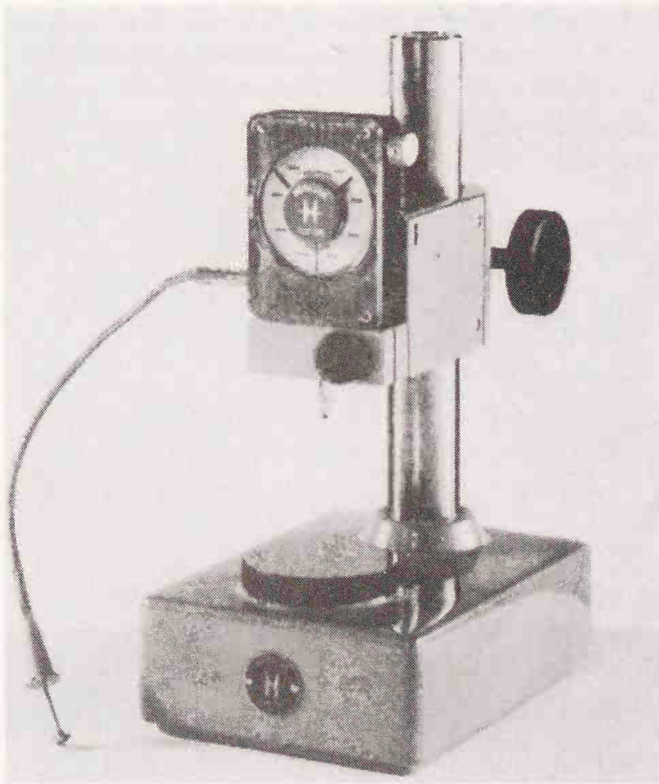
Figure 2-16 A precision dial comparator. This instrument is direct reading to 0.00005 inch. (Courtesy Hamilton Watch Company.)
