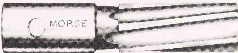
Figure 10-11 Stub screw-machine reamer. Available in decimal sizes from 0.0600 to 1.010 inch inclusive. Regularly furnished with right-hand cut and 7^\circ left-hand helix. (Courtesy Morse Twist Drill & Tool Company.)
