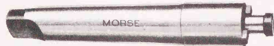
Figure 14-9 A shell-end-mill arbor with tanged end. (Courtesy Morse Twist Drill & Machine Company.)
