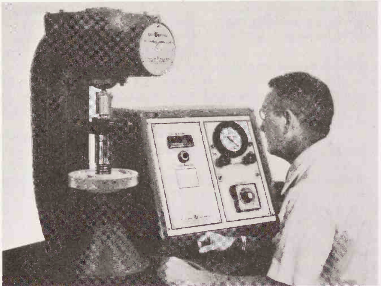
Figure 3-4 Air-o-Brinell metal hardness tester with Digito-Brinell system for digital readout of Brinell values. (Courtesy Tinius Olsen Testing Machine Company.)
