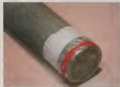
A simple mold made of 3" PVC pipe from the hardware store. The end is sealed with plastic wrap which is both taped and rubber banded - you really do not want to have the plastic wrap come off before you are ready.
