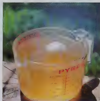
The strength of the lye is tested by floating an egg: if the egg sinks, the lye solution is weak and it would be added to more ash to make a more concentrated solution.
