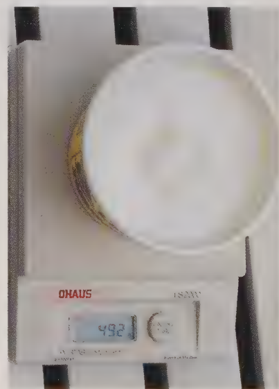
One of many suitable types of digital scales. This scale has a tare function and is weighing a container of lard.
