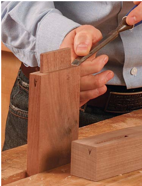
Undercut tenon shoulders. Use a chisel to cut a slight downward bevel (no more than \frac{1}{32} in.) on the tenon shoulder.
