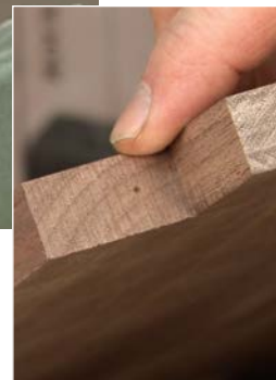
Tap once. A light mallet tap drives the dowel center into the shelf edge (above). The dimple (right) locates the drill bit for a perfectly aligned hole.
