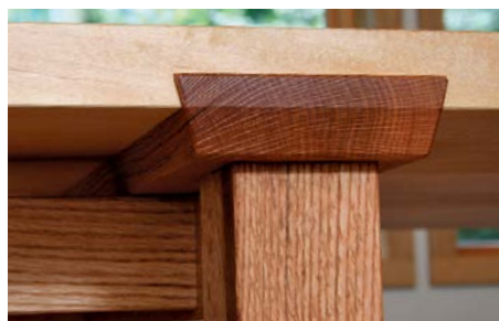
Flat cleat. Simply a board with beveled edges, this cleat is easier to make than the shouldered version, but can't be very tall. It works well with a base that has four legs.
