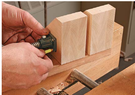
Add the swivel face. Screw the threaded rod through the guide to see where to attach the swivel face to the sliding jaw.
