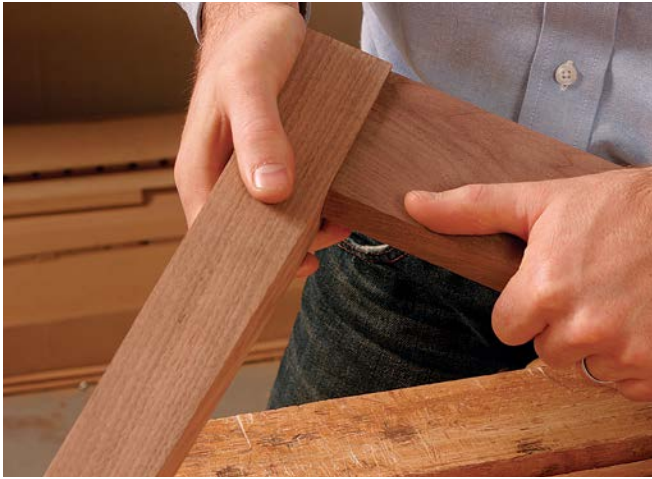
Gap-free table legs. Undercutting is an efficient method for improving the fit of a mortise-and-tenon joint.
