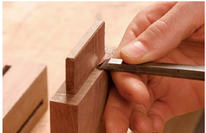
Carry the bevel around the shoulder. Work your way around the perimeter of the tenon, leaving the outermost edge intact.
