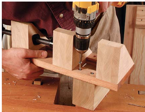
Screw on the bench block. A block of wood, screwed to the two rails of the base, holds the miter shoot in a bench vise.
