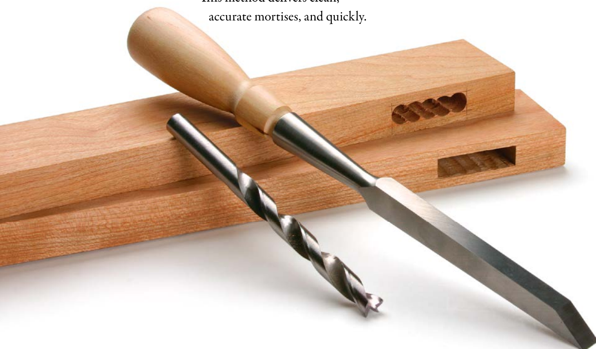
Mortises in no time. Drill out the waste, then use a unique chiseling technique to handle the rest.
