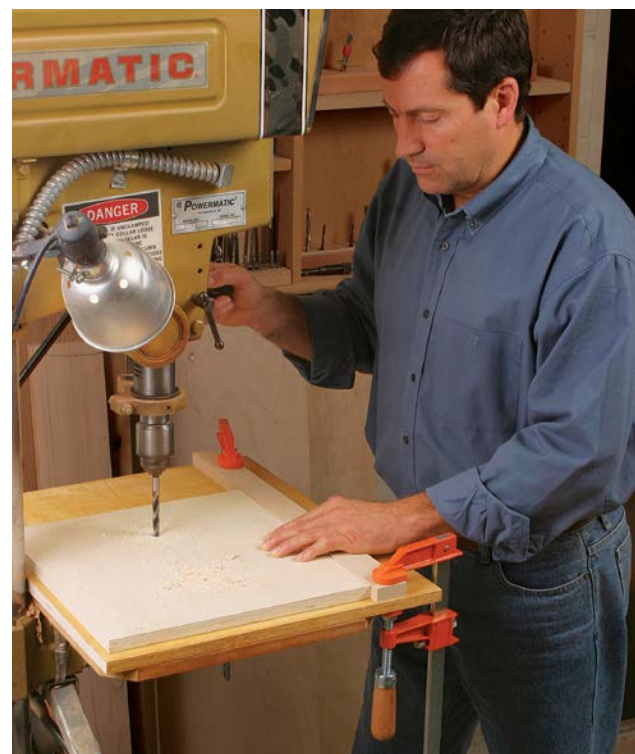
Locate the circles on the front plate. Drill two \frac{3}{8} -in. holes on the centerline for the circles' center holes. Use a fence to ensure that the holes are aligned.
