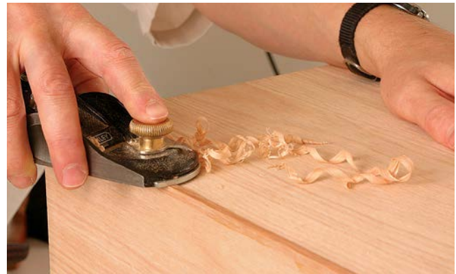
A solid-wood corner. Plane and sand the strip of wood flush with the veneered sides. The corner can then be slightly rounded without risk of cutting through the veneer.
