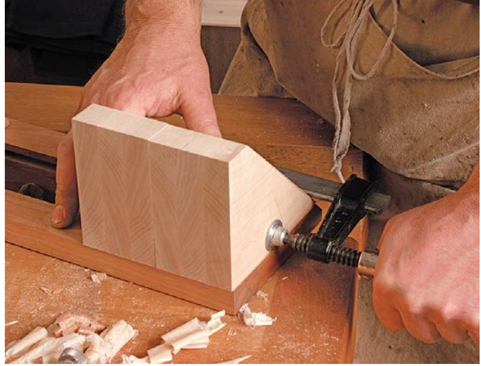
Attach the sliding jaw. After you have screwed the fixed jaw to the base, clamp the sliding jaw to the fixed jaw and screw it to its sliding spacer.
