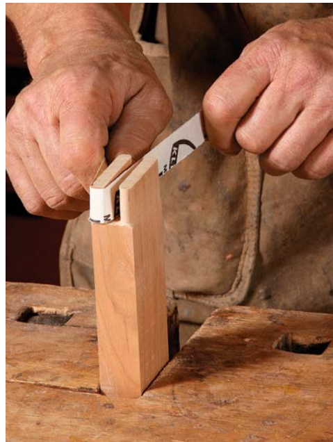
Round the tenons. Sandpaper used with a shoe-shine stroke makes quick work of knocking the corners off the tenons so they fit the rounded corners of the routed mortises.
