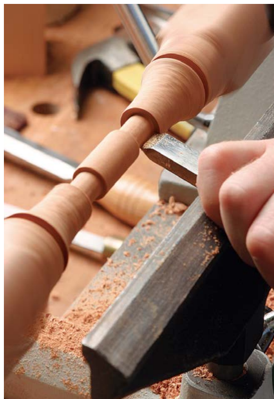
One-touch technique. Use a skew chisel to undercut a pull while it is still on the lathe.
