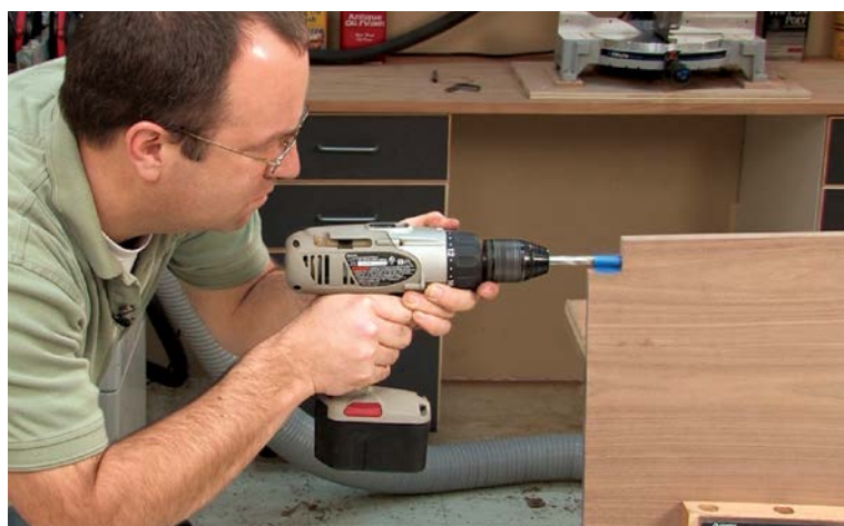
Locate the shelf. A support block clamped to the leg holds the shelf in place.
