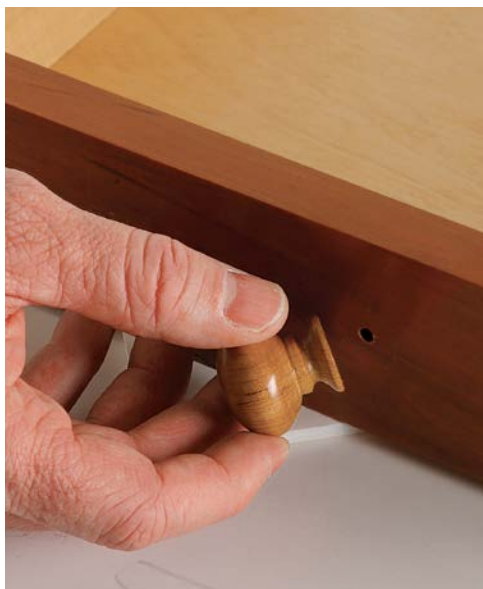
Flush mount. Pulls should sit flush against a drawer front.
