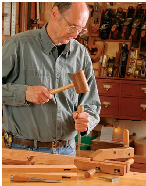
Mortises in no time. Drill out the waste, then use a unique chiseling technique to handle the rest.
