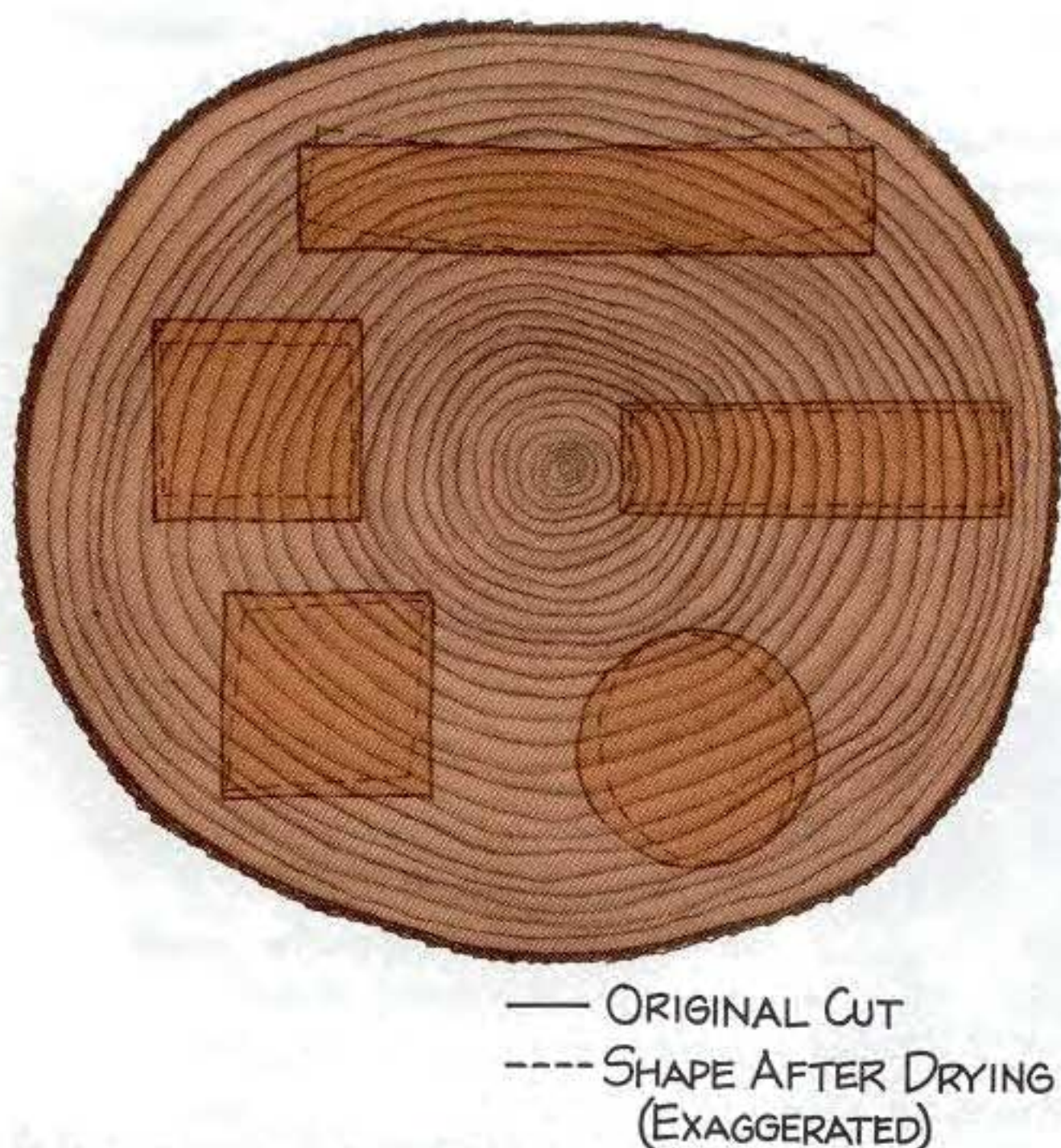
1-10 Because the radial and tangential movement of wood is uneven, boards tend to deform as they go through an annual moisture cycle. The way a board will deform depends on how it is cut from the tree.
