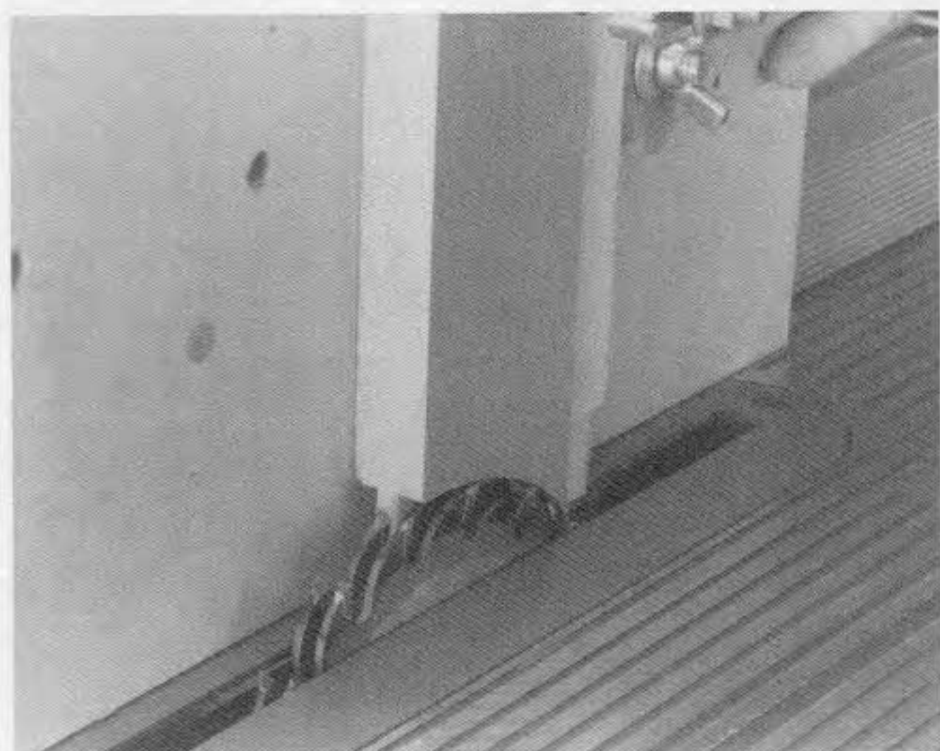
5-15 To cut a tenon with a dado cutter, mount the workpiece in a tenoning jig. Back up the workpiece with a scrap board to prevent the cutter from tearing the wood grain when it exits the workpiece. Then guide the jig along the fence, past the cutter.
