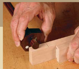
MARK MORTISES AND TENONS AT THE SAME SETTING. Fill in the scribed lines with pencil marks, so the lines are easier to read.
