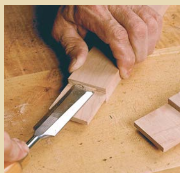
FINE-TUNE THE FIT. Rasps and chisels are good choices for removing material from either the tenon or the mortise. Hand-cut frames need many test runs before you can call them done.
