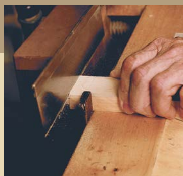
CUT THE SHOULDERS WITH A DOVETAIL SAW. For well-fitting joints, make sure that you cut to the same line on all the pieces.
