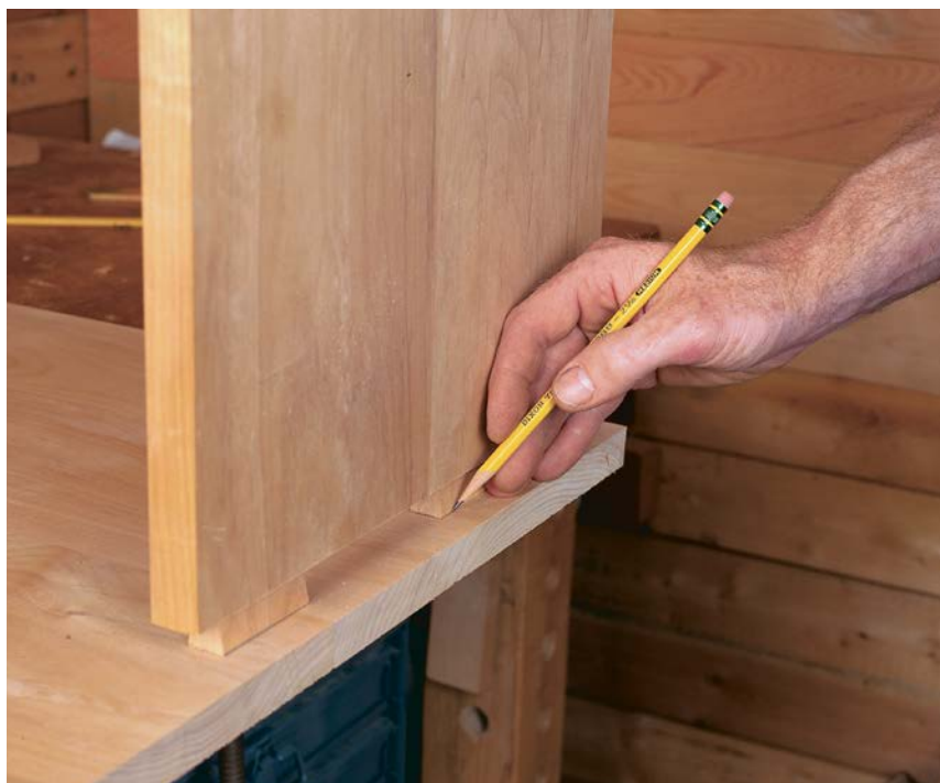
MARK THE DOVETAIL SLOTS FIRST. The locations for dovetail slots in the top of the lower cabinet are marked directly from the dovetailed keys.
