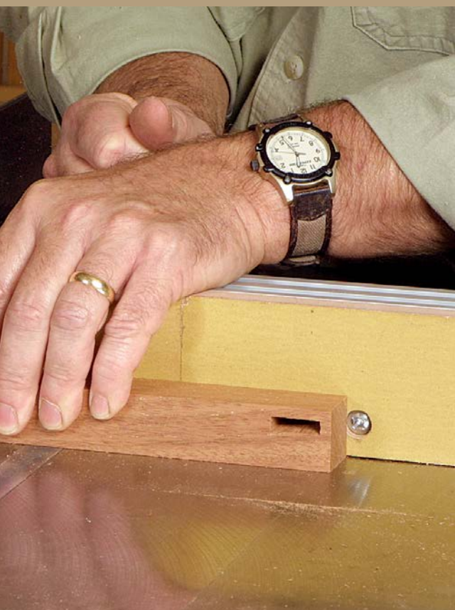
ROTATE THE WORKPIECE to cut the adjacent miter. The mortise that was facing the surface of the tablesaw should be facing the miter gauge on the second cut.
