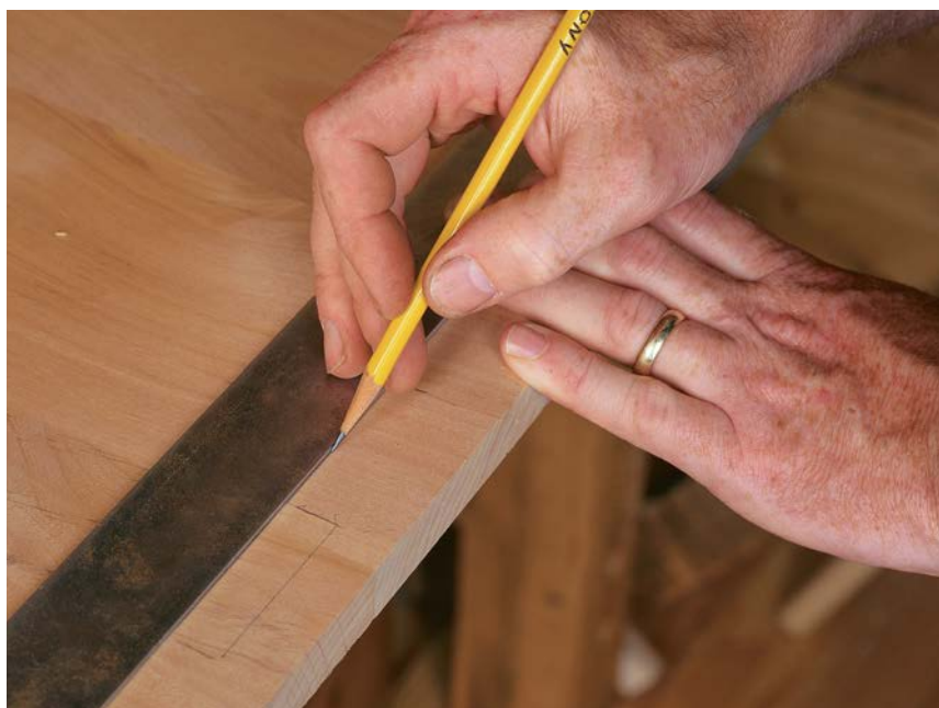
LAYOUT THE ESCAPEMENTS using the dovetail slots as a guide. When you cut the joints, remember that the escapements are at the back of the cabinet.
