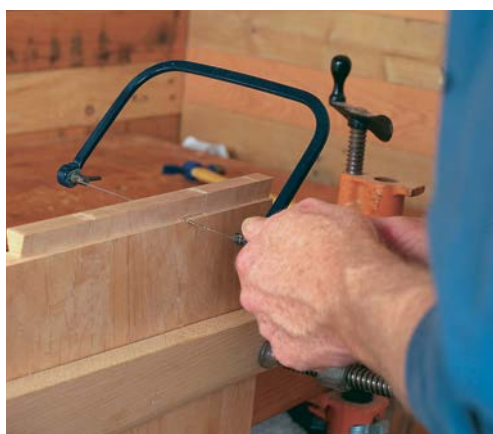
AFTER CUTTING A DOVETAIL the full width of the upper case side, cope out the dovetail keys (left), and then clean up the shoulder with a chisel (below). Pare carefully: The line of the finished joint depends on the flatness of the shoulder.
