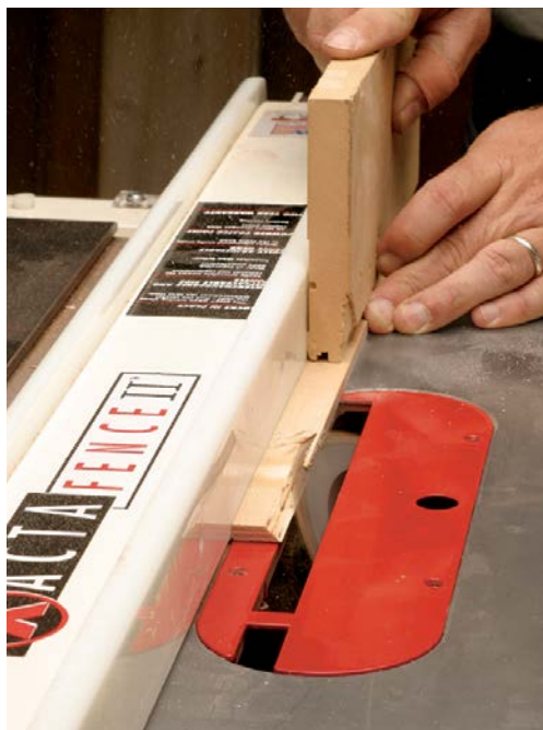
CUT THE TENONS from a long strip of material. Cut a bevel along one edge of the tenon stock. Then bevel one end and crosscut to length.
