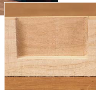
DEDICATED SLOT MORTISER Chris Becksvoort cuts a slot for a mortise lock in a finished door. Unlike a router, a dedicated slot mortiser is quiet and a simple pleasure to use.
