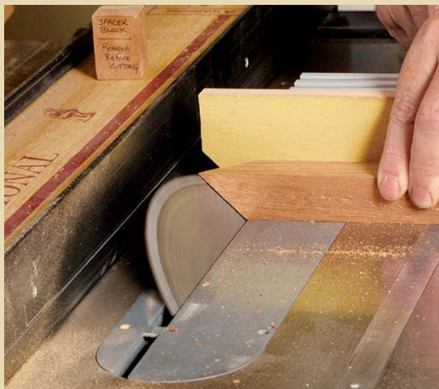
ROTATE THE WORKPIECE to cut the adjacent miter. The mortise that was facing the surface of the tablesaw should be facing the miter gauge on the second cut.
