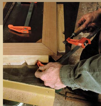
NO BAND CLAMPS HERE. Because the spline extends beyond the outside corner, it is necessary to use block clamps.
