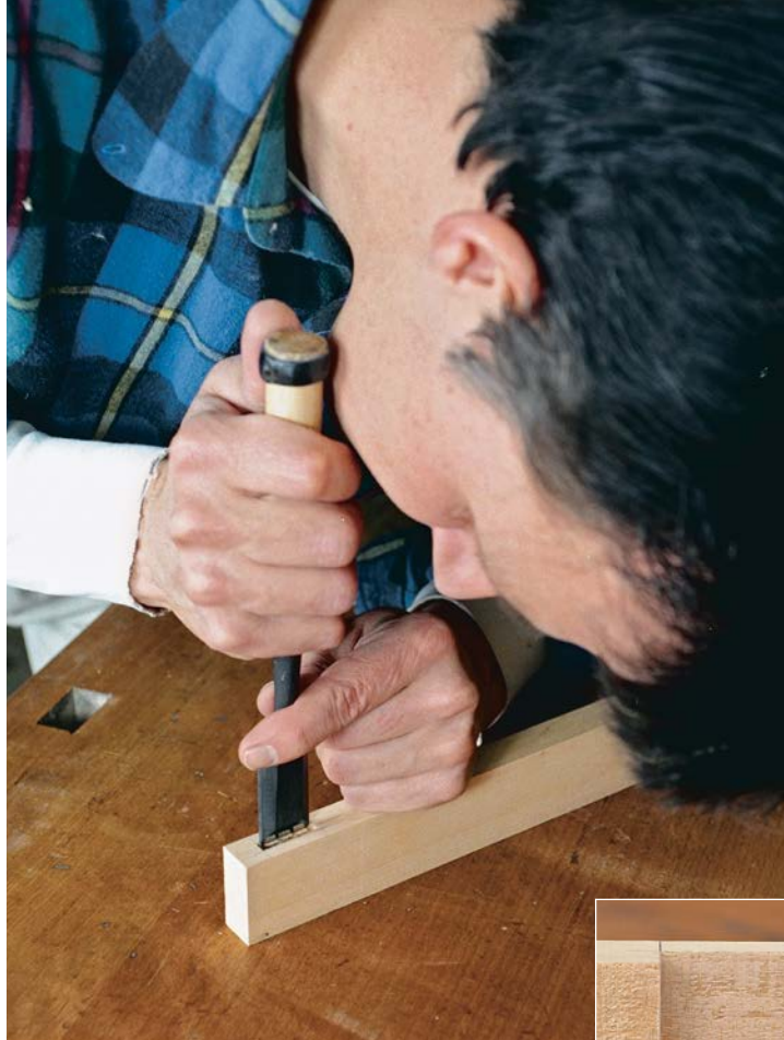
DRILL AND PARING CHISEL. Carl Swensson uses a drill press to quickly hog out the mortise waste (above), then a paring chisel to shave off the ridges left by the twist drill. Easy to see, the ridges make excellent guides for paring the mortise cheeks square and flat.
