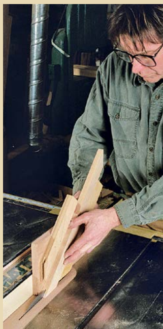
CUT ONE END. Hold the workpiece firmly in place and register the jig against the tablesaw fence.
