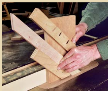
CUT ONE END. Hold the workpiece firmly in place and register the jig against the tablesaw fence.
