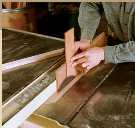
CUTTING THE SPLINE. Use a tenoning jig to trim the spline to thickness.
