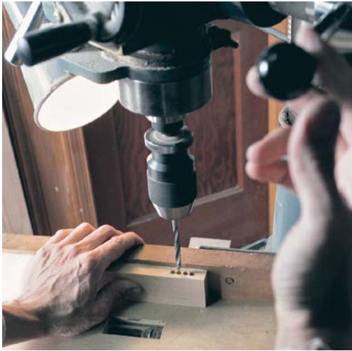
DRILL AND PARING CHISEL. Carl Swensson uses a drill press to quickly hog out the mortise waste (above), then a paring chisel to shave off the ridges left by the twist drill. Easy to see, the ridges make excellent guides for paring the mortise cheeks square and flat.
