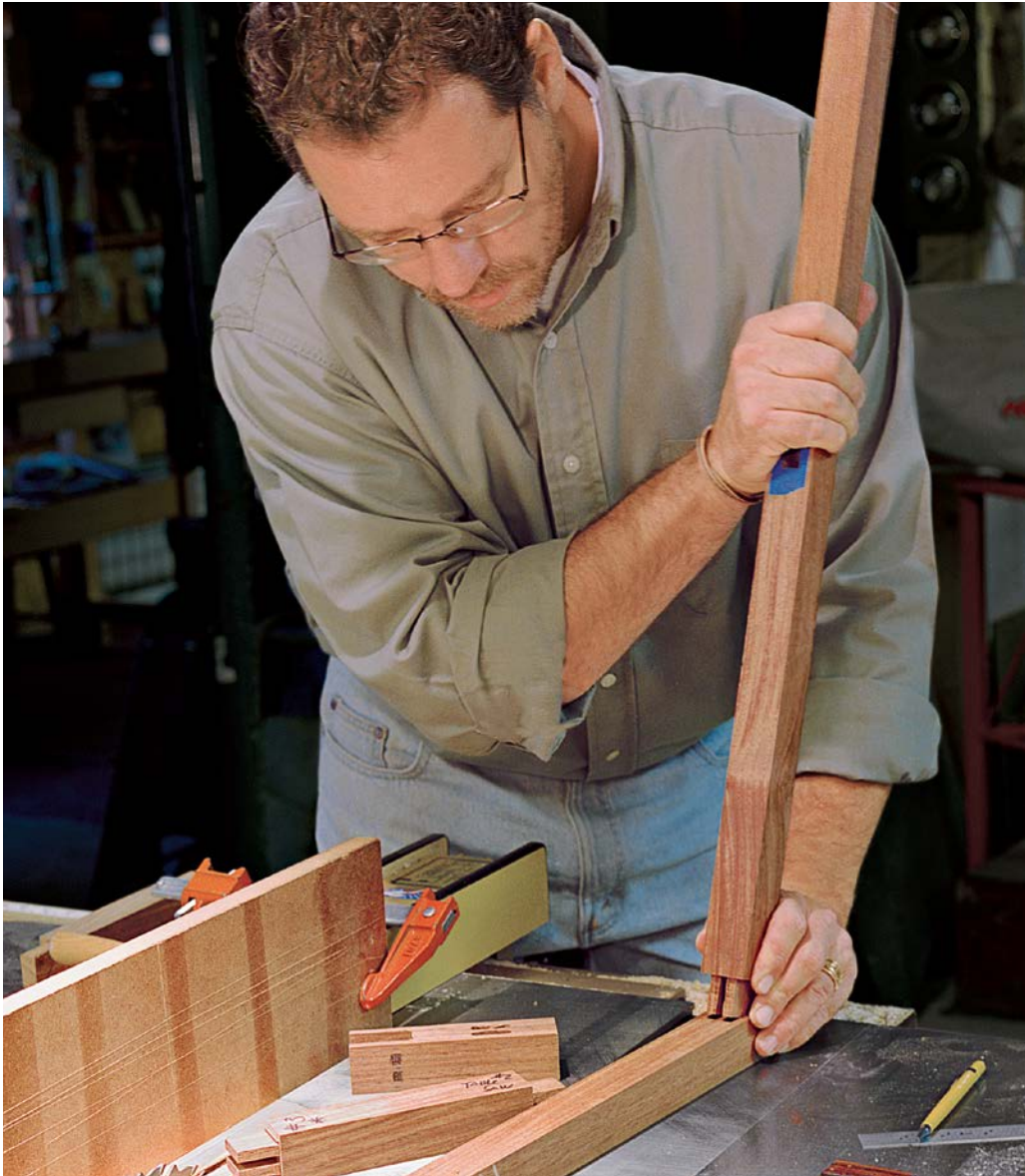
TOOLS FOR MULTIPLE MARKING. A story stick and a marking knife add accuracy and reliability to a repetitive process.
