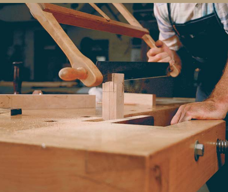
THE BOWSAW is Klausz's tool of choice for cutting this joint by hand because the long, wide blade tracks well and cuts quickly.
