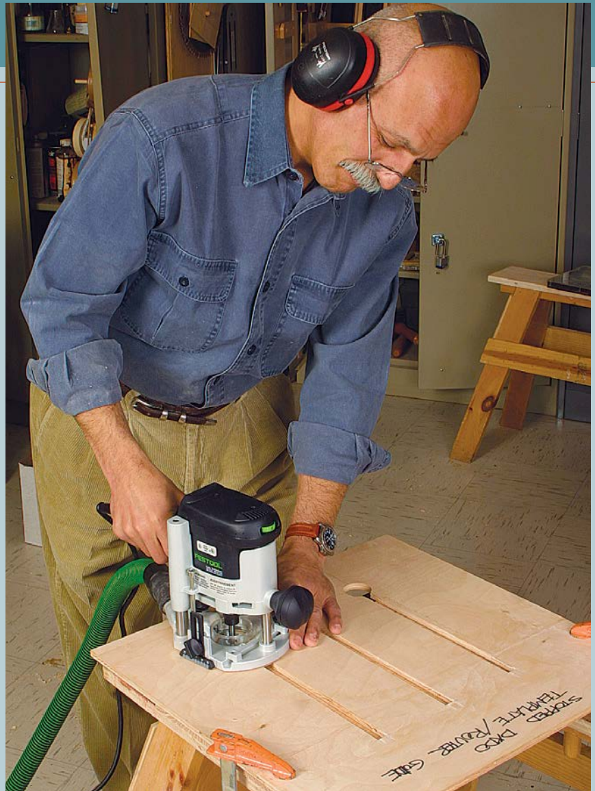
THE TEMPLATE GUIDES THE ROUTER. A rub collar (or template guide) screwed to the router base runs against the template, guiding the router bit.
