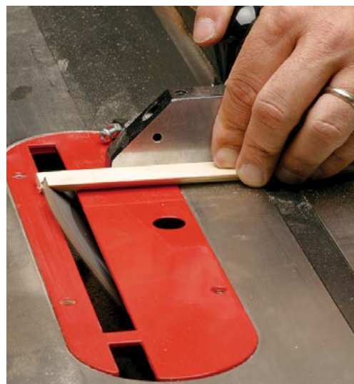
CUT THE TENONS from a long strip of material. Cut a bevel along one edge of the tenon stock. Then bevel one end and crosscut to length.
