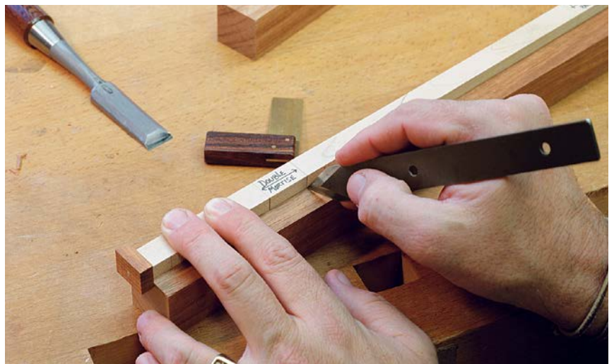
TOOLS FOR MULTIPLE MARKING. A story stick and a marking knife add accuracy and reliability to a repetitive process.
