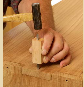
SHOPMADE TOOL for squaring holes. Janofsky uses a thin, square bar of steel, tapered on a bench grinder, to square the holes. The wood block makes the tool easier to hold.
