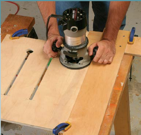
CUT THE TEMPLATE GUIDE. With a T-square guide clamped to the edge of the plywood template, rout a slot for the template guide to ride in.
