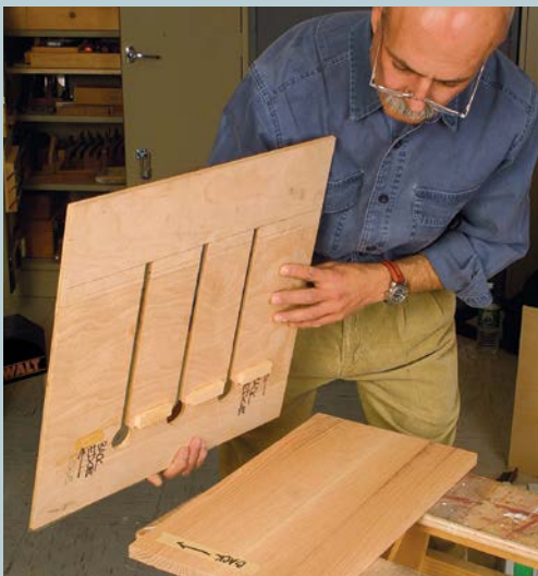
ROUTER TEMPLATE SPACES PARTITIONS EVENLY. Because the stopped dados for the partitions must be cut precisely and in identical positions on both the upper shelf and the top, it is best to use a plywood template to guide the router.
