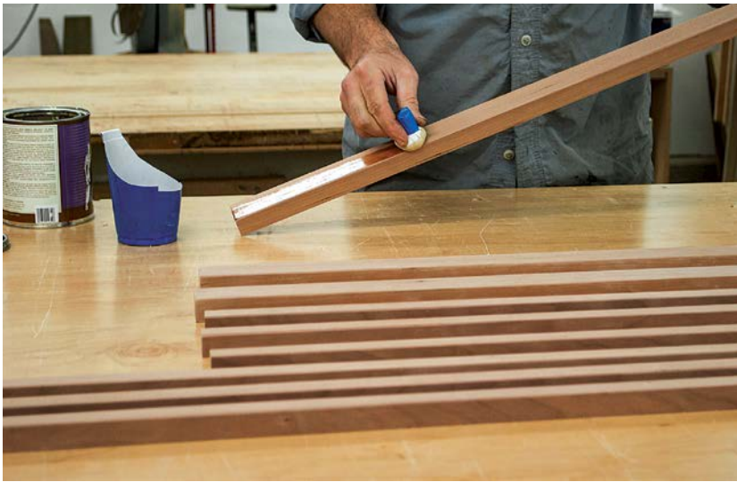
Apply oil to the parts in long, even passes using a wad of gauze wrapped in a scrap of a T-shirt.
