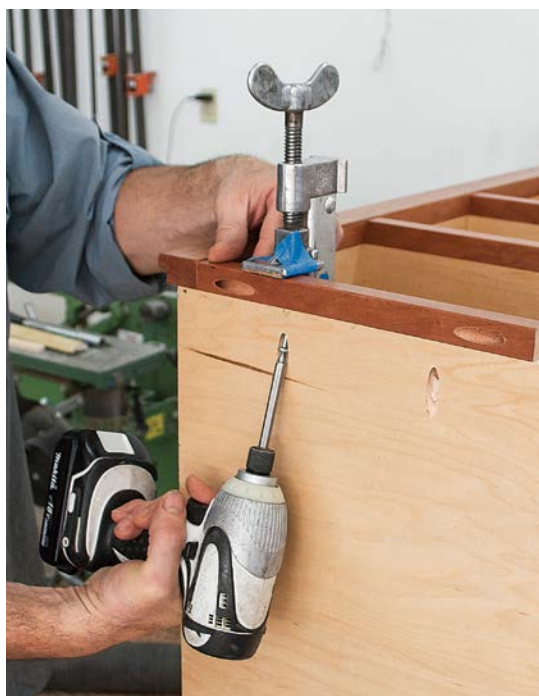
Flip the cabinet onto its back to access the pocket holes on the bottom when installing the last horizontal drawer frame piece.
