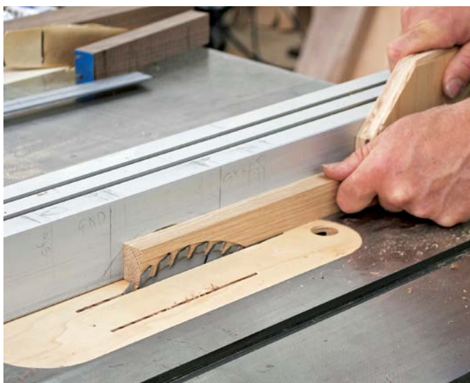
Cutting a shallow dado on the underside of the handle bar gives a positive grip when opening the drawers.
