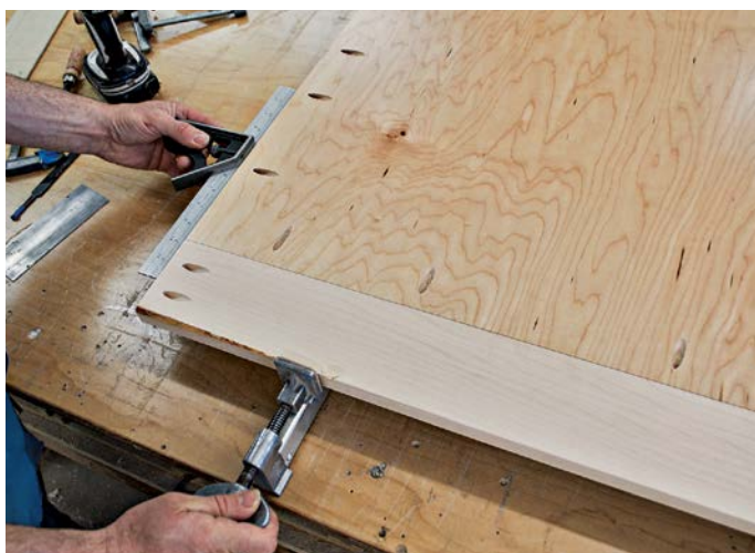
Clamp the bottom panel rail to the plywood end panel, and flush up the edge with a straightedge.
