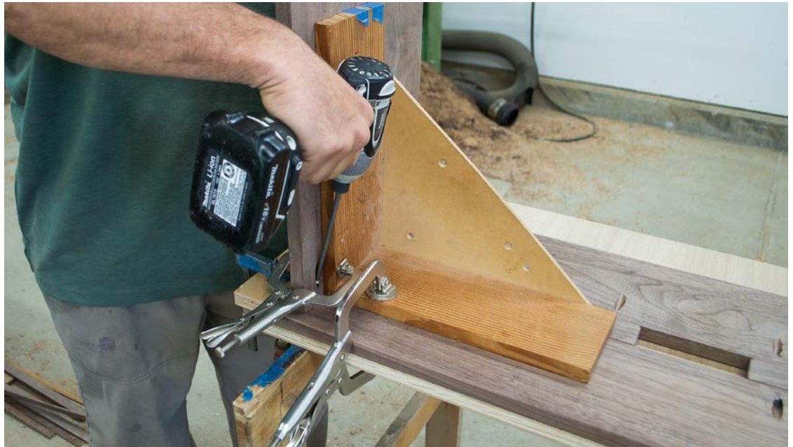
A right-angle jig clamped to the workpiece (and bench) helps to hold the piece upright during assembly.
