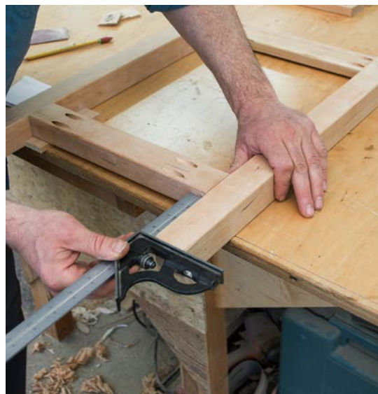
Use a square to locate the lower stretcher on the legs.
