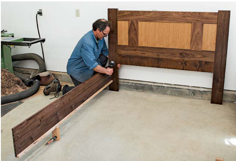
A block of wood helps to support the mattress rail as you attach the other end to the headboard.
