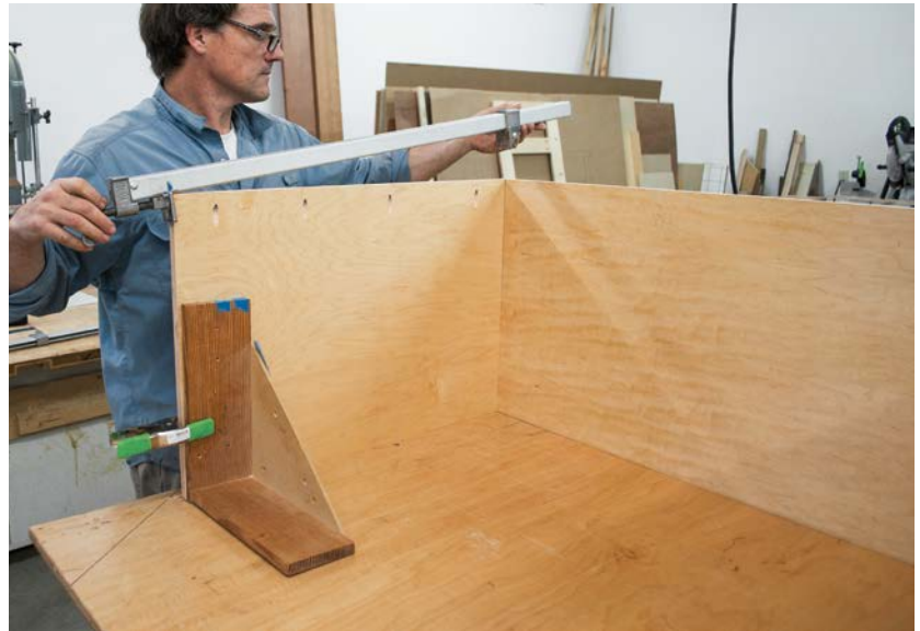
Use the right-angle jig to help support the plywood pieces when attaching the clamps.
