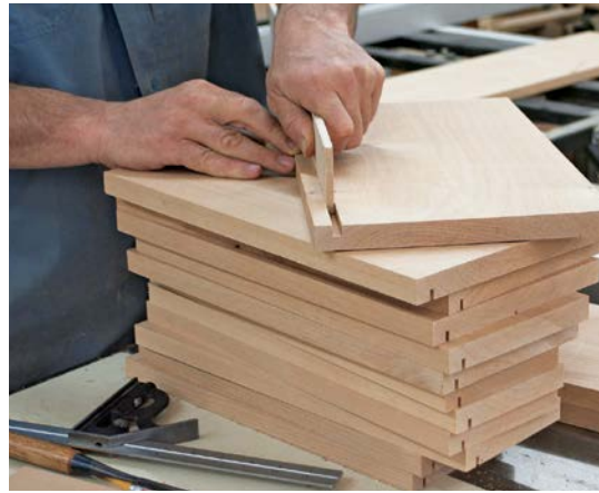
Check that the groove for the drawer bottom is not too tight.
