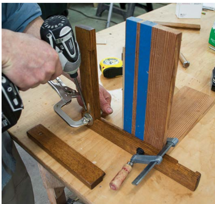
Use the right-angle jig to hold the top rail of the picture frame while driving the pocket screws from the stile.
