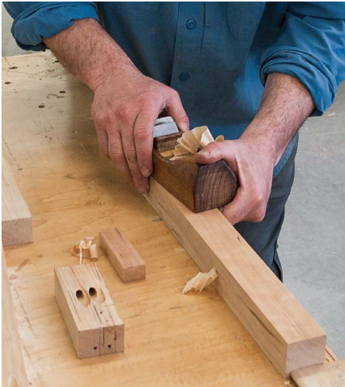
Nothing gets rid of machine marks faster than a sharp handplane.
