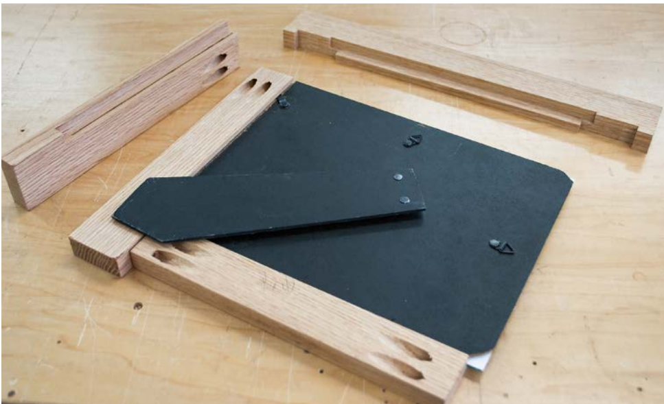
Use a chisel to square off the end of the stopped rabbets.
