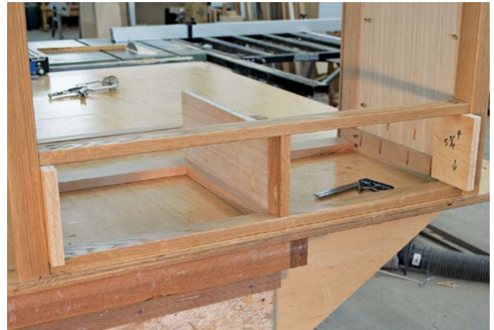
With the 5 \frac{3}{4} -in. jig spacers on either side, set the #1 horizontal drawer divider on top with the pocket holes facing up.
