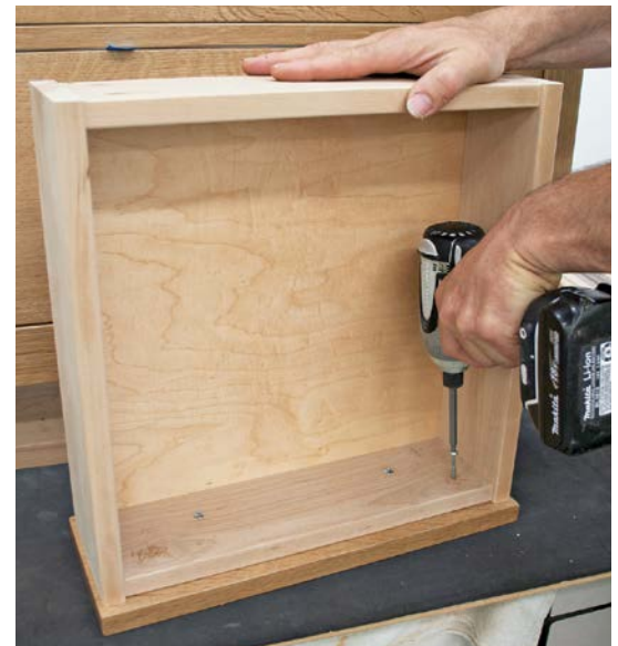
Predrill and drive pocket screws through the drawer into the drawer front.
