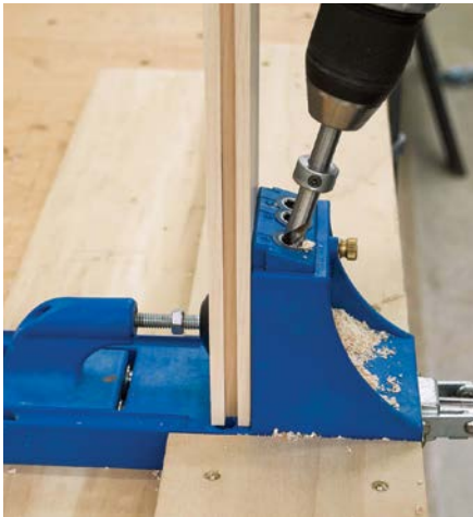
Drill the back-panel rails with the adjusted drill bit and jig.
