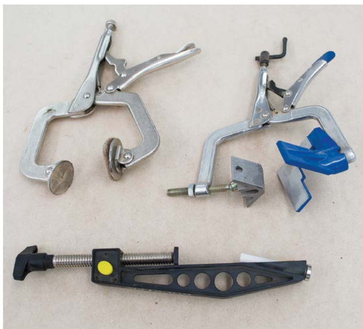
Clamps are essential for pocket hole joinery. Shown here (clockwise from top) are a face clamp, a 90-degree corner clamp, and a Rockler® Pock-it Hole Clamp® with Quick Release.
