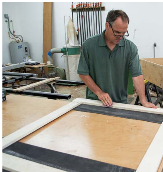
Lightly sand the inside edge of the frame to soften the step between the frame and plywood sides.
