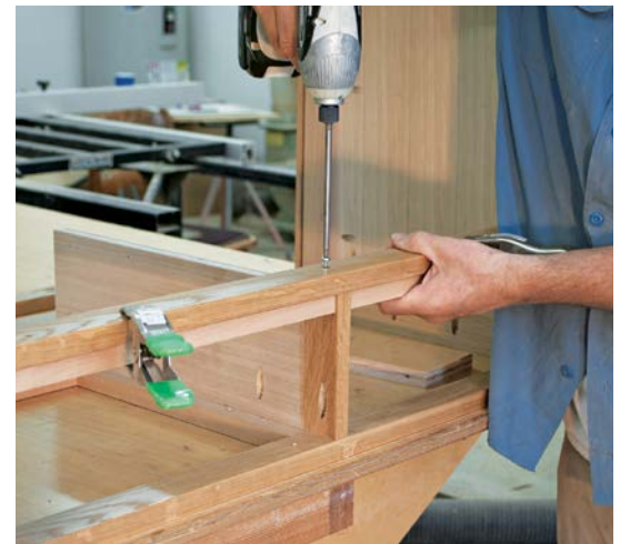
Drive a pocket screw through a countersunk hole on the underside of the frame into the top drawer partition.
