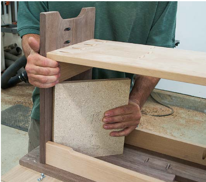
Hold the upper spacer in place as you slide out the lower spacer to keep from scratching the top of the shelf.
