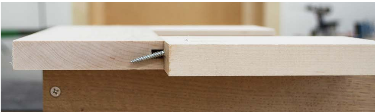
Using longer screws and the \frac{1}{2} -in. thickness setting ensures a stronger connection.
