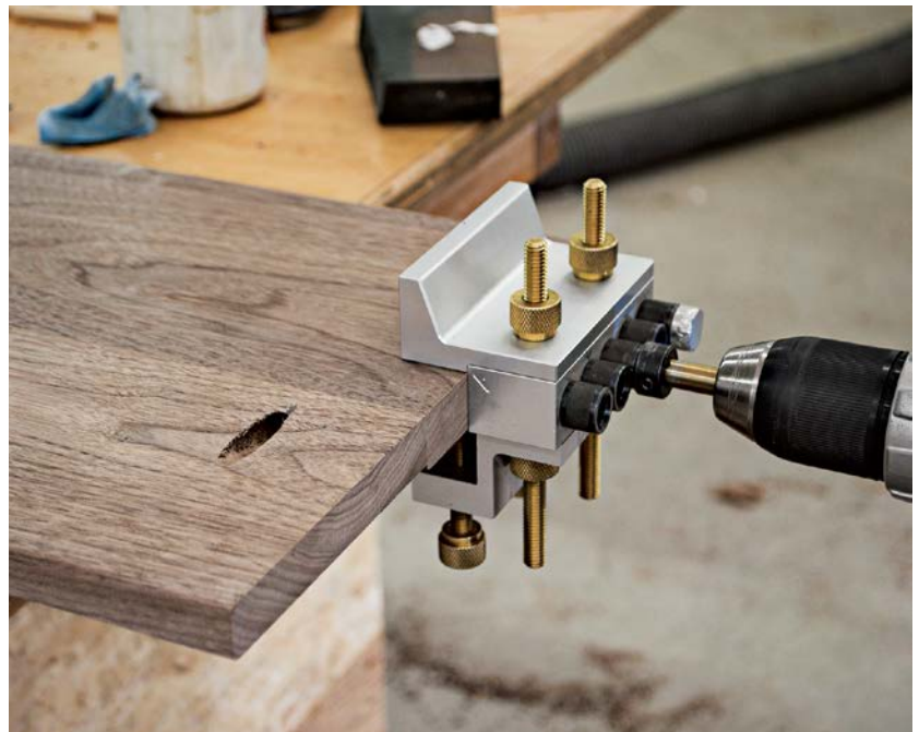
With the index pin set in the first pin of the doweling jig, drill for dowels in the third and fifth hole in the mattress rail.
