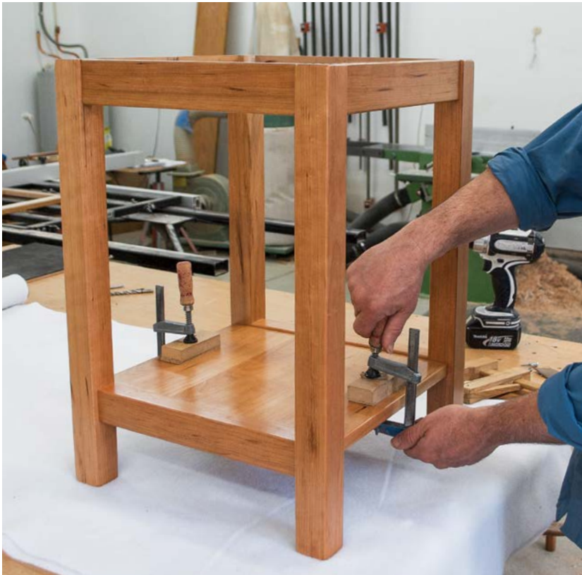
Clamp the shelf in place using protective cauls against the finished surface.
