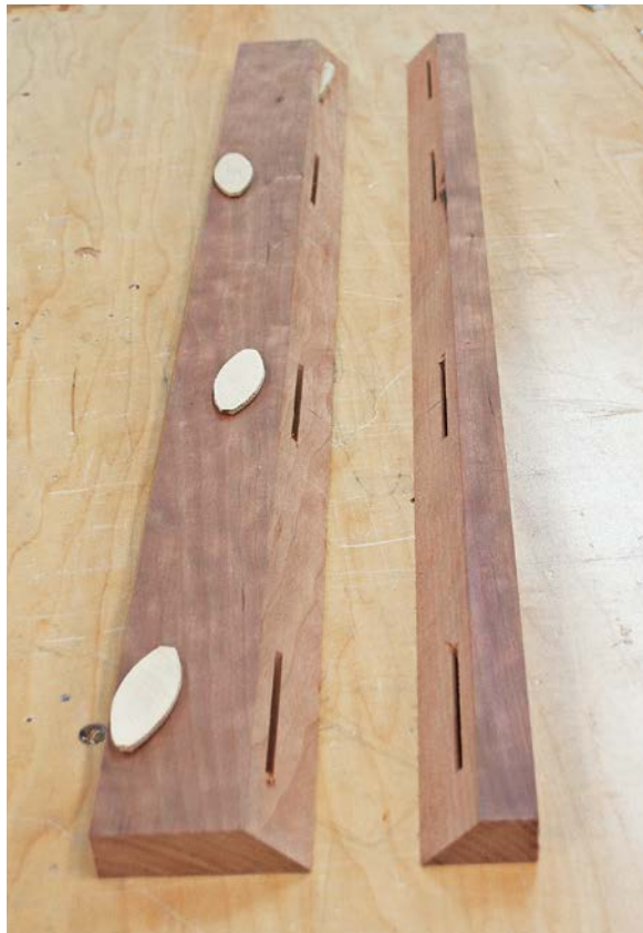
Four biscuits down the length of the corner posts help keep it aligned during glue-up.
