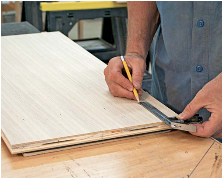
Lay out the location of the pocket holes next to the biscuits. Make the mark high enough so that it can be seen over the pocket hole jig.
