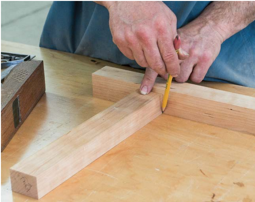
Mark the stretcher location on the legs to help you know where to stop and start the roundover edge on the leg.
