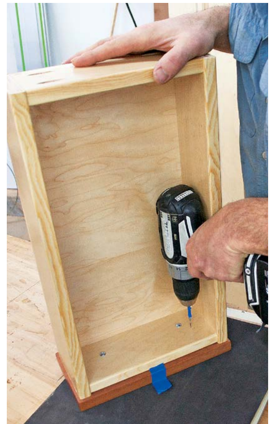
Thread the #8-32 screws into the plastic plug locaters in the drawer front (left), then add two pocket screws to secure the drawer front in its final location (above).
