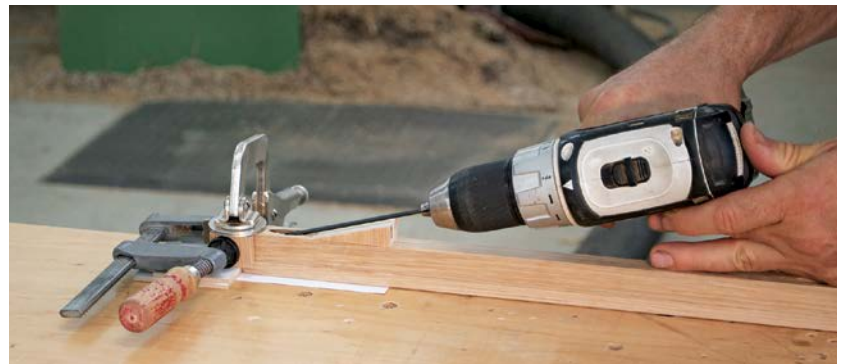
Pre-drill the end blocks of the handle using a 15-degree gauge, shimming up the handle bar with card stock so that it is flush with the end block. Clamp across the end block and hold in place with the face clamp.
