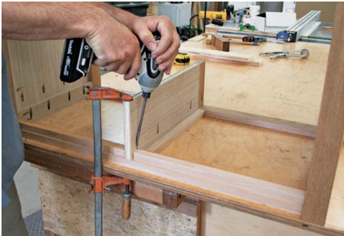
Use spacers on either side of the top drawer partition to center it during installation.
