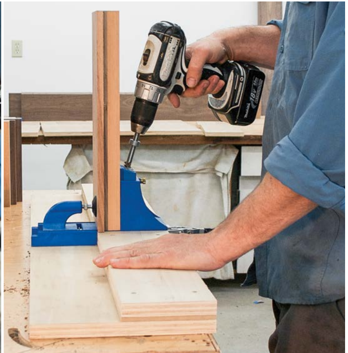
Use the portable pocket hole jig to drill the pocket holes in the rails (left). The stiles are short, so it's easier to use the benchtop jig for these (right).
