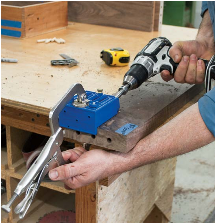
Use the portable pocket hole jig to drill the pocket holes in the rails (left). The stiles are short, so it's easier to use the benchtop jig for these (right).
