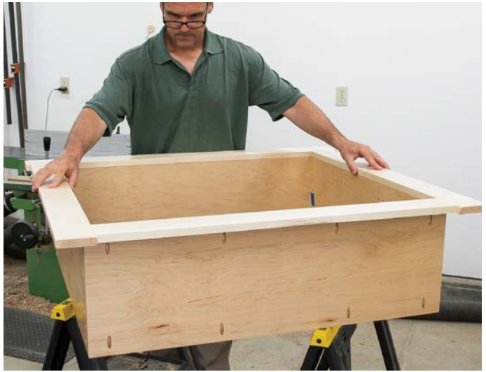
With the front frame assembled, check the fit on top of the cabinet. It should just barely overhang the plywood core.
