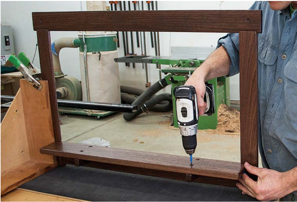
Predrill the shelf and corbel before driving the screw.
