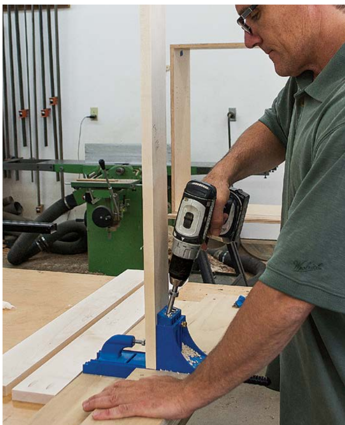
Drill the bottom rail with pocket holes on both ends after drilling the top ends of the stiles.
