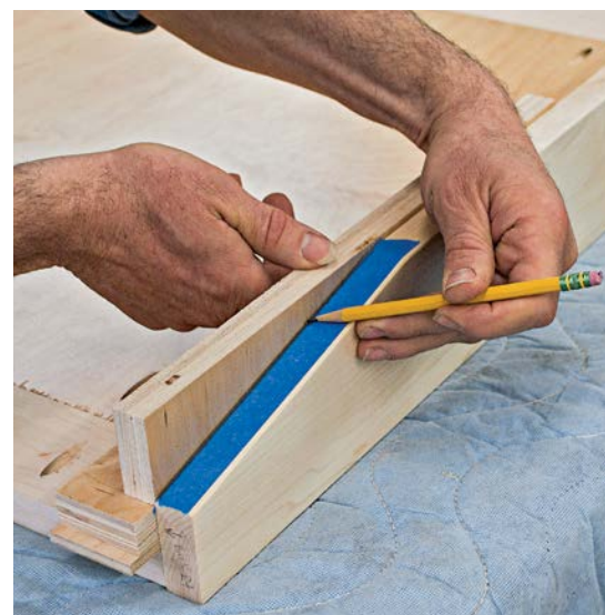
Raise the furring strip by about 1 in. to trace the slope of the corner post.
