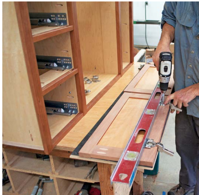
Use a straightedge against the Euro hinges to help align them when drilling the screw holes.
