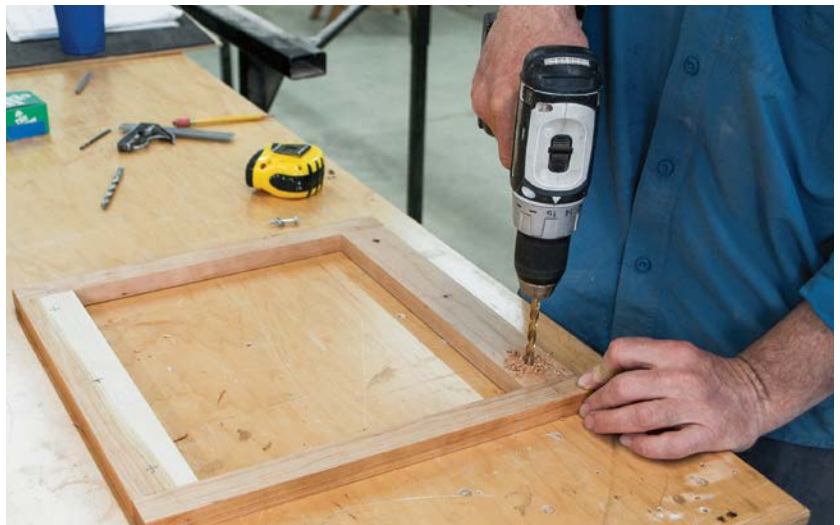
Drill oversize holes in the spacer frame to allow for wood movement of the top at the edges.
