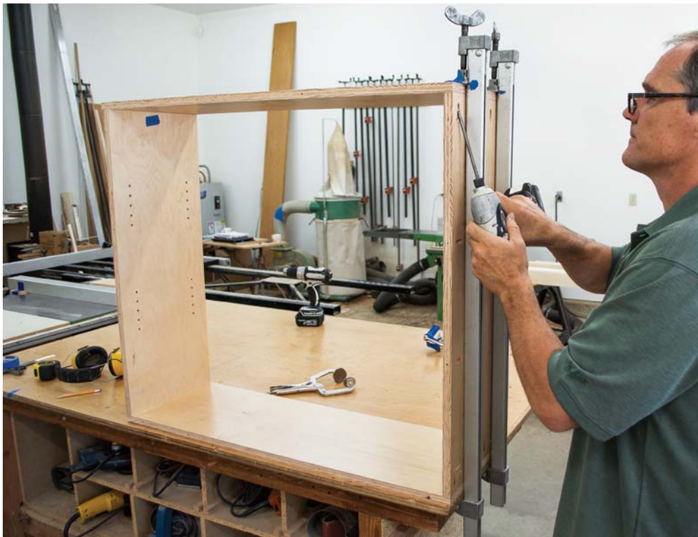
Use bar clamps to hold the top panel in place while screwing.
