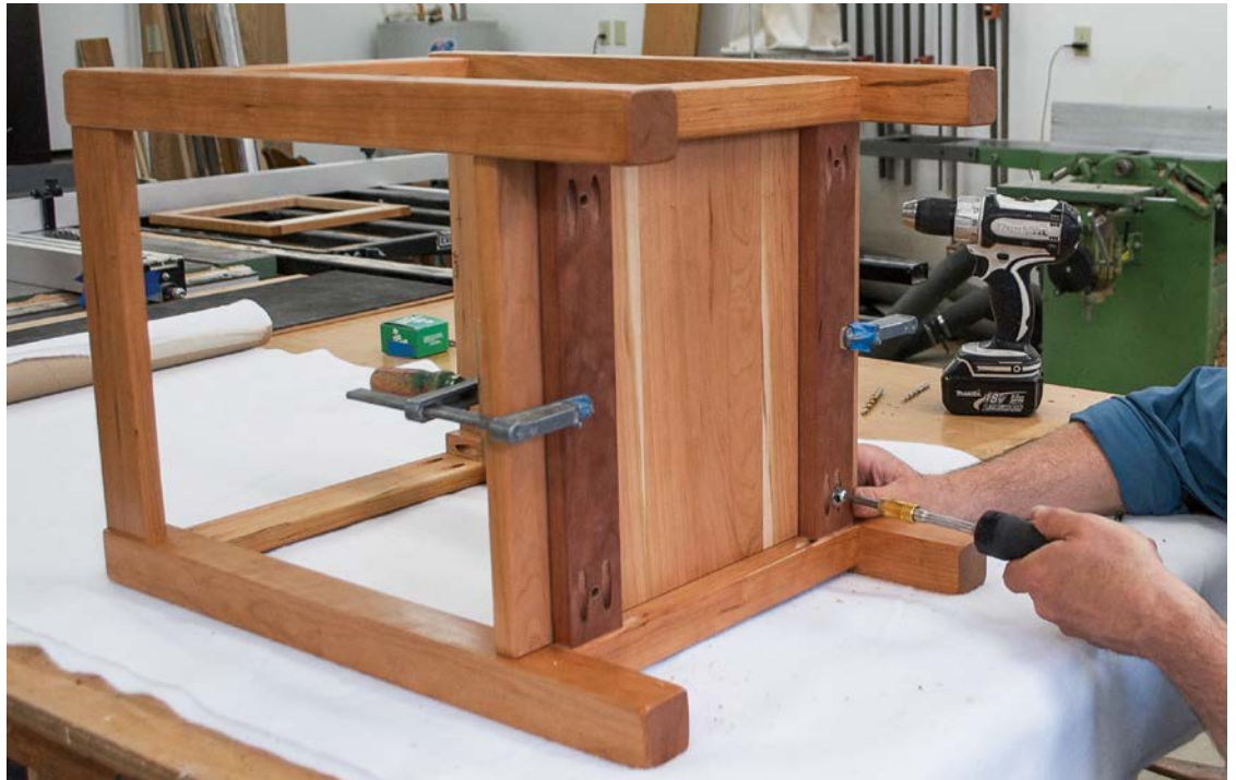
Clamp the shelf in place using protective cauls against the finished surface.
