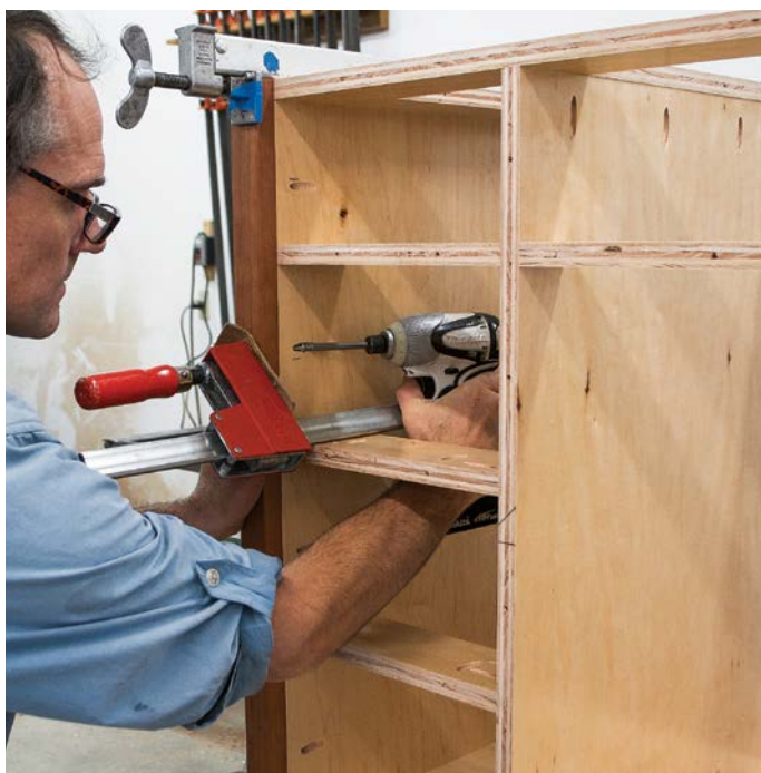
Attach the end vertical face frame with clamps, then drive pocket screws from the inside.
