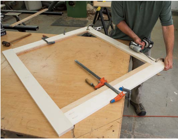
Using the vertical spacers as locating jigs, attach the bottom rail with pocket screws and face clamps.
