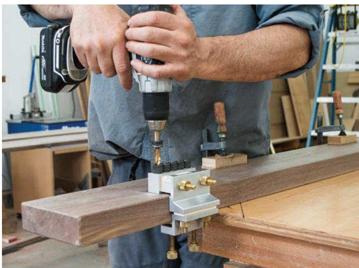
When drilling the post for the dowels, use a 1-in. spacer in the doweling jig to align the mattress support rail location onto the post.
