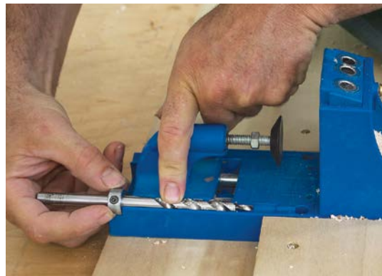
Change the stop collar setting to \frac{1}{2} in. for drilling the rails for use with 1\frac{1}{2} -in. screws.
