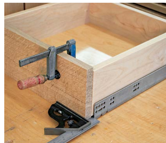
Press the drawer slide onto the drawer, and with the drawer front against the drawer box, measure the distance to the front of the slide.
