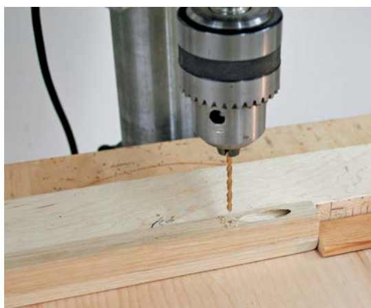
Cutting a shallow dado on the underside of the handle bar gives a positive grip when opening the drawers.
