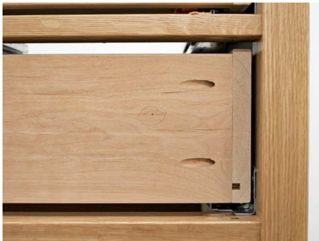
A small point locates where the \frac{3}{16} -in. hole should be drilled.
