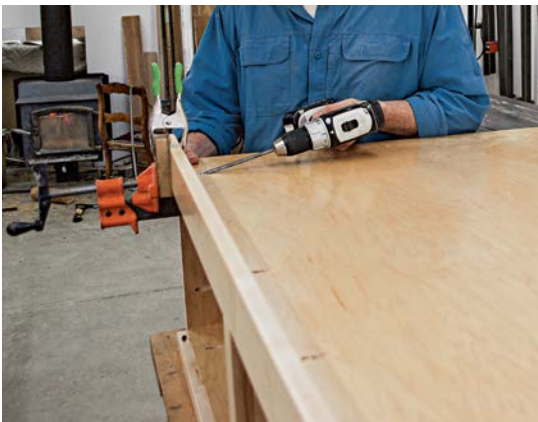
Use wide bar clamps to hold the top face frame rail to the plywood top.
