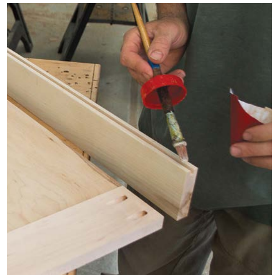
Begin the back-panel assembly with the rails and panel dry-fit, and apply glue to the joint between the stiles and the rails.
