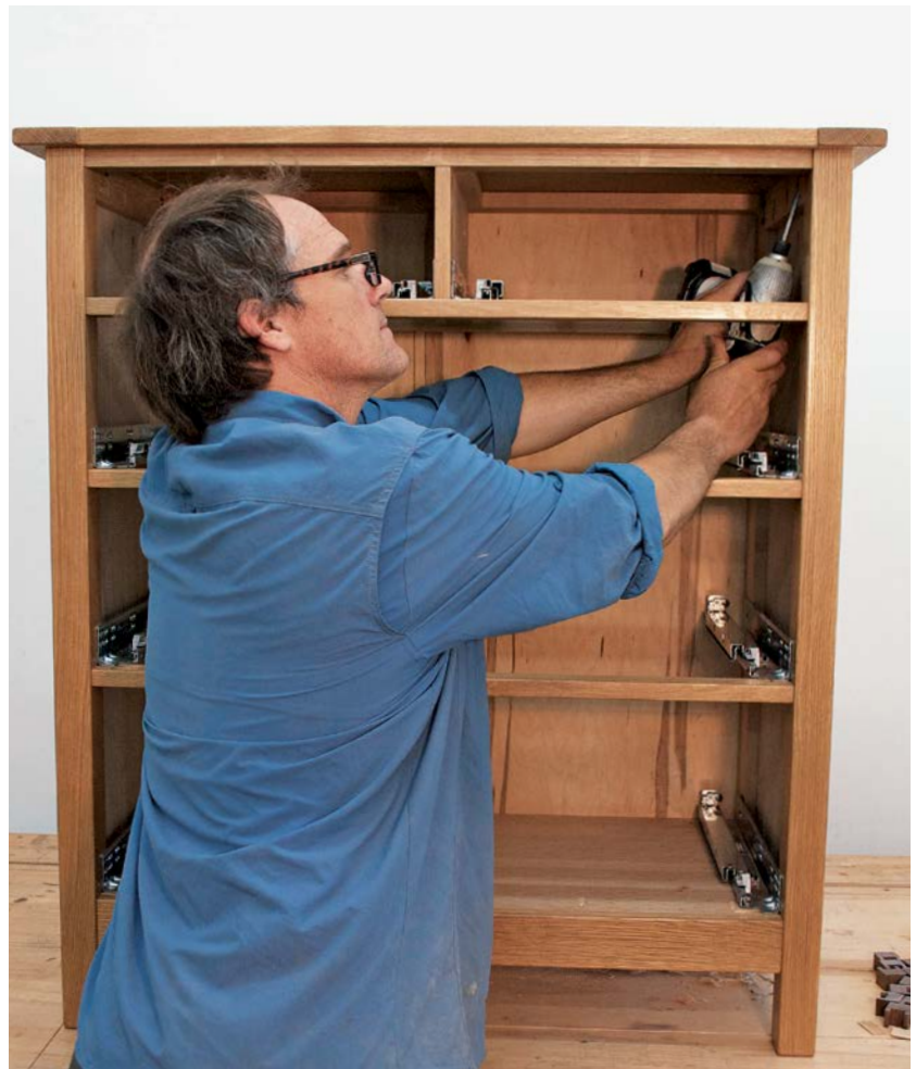
Drive pocket screws through the top rails on the side panels into the breadboard ends.
