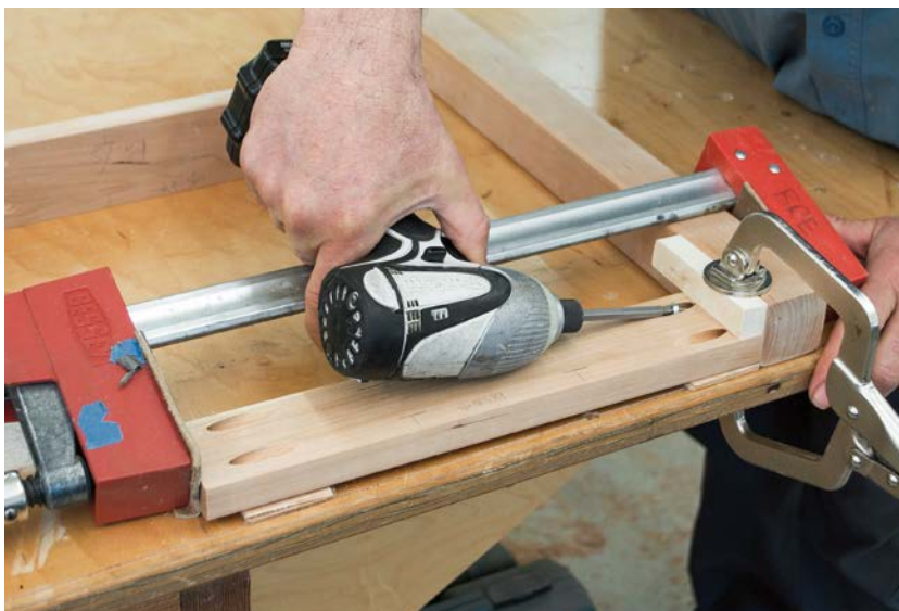
Use a bar clamp and a face clamp to hold the leg/skirt assembly in place while driving the pocket screws.
