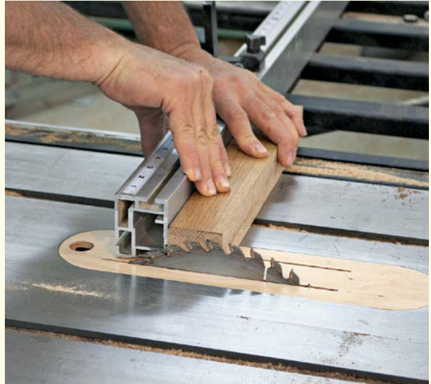
Removing just a small amount of wood below the surface makes it easier to pare the rail to fit.
