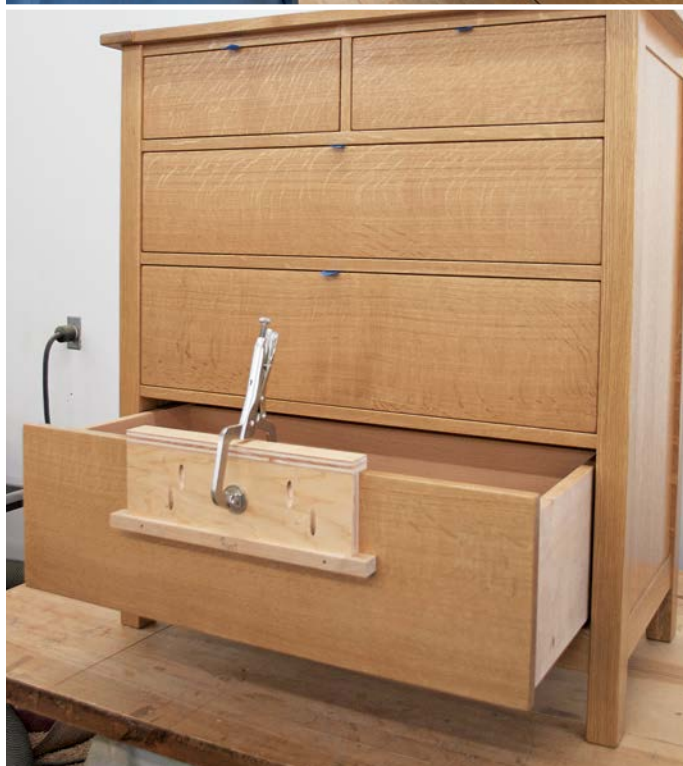
Attach the drawer jig to the drawer with the face clamp, then drill out for the handles.
