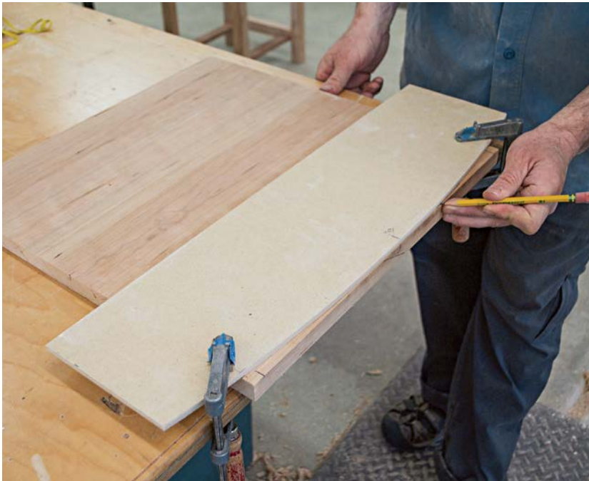
Align the template on the tabletop so that the center and end marks correspond. Trace the outline onto the top.
