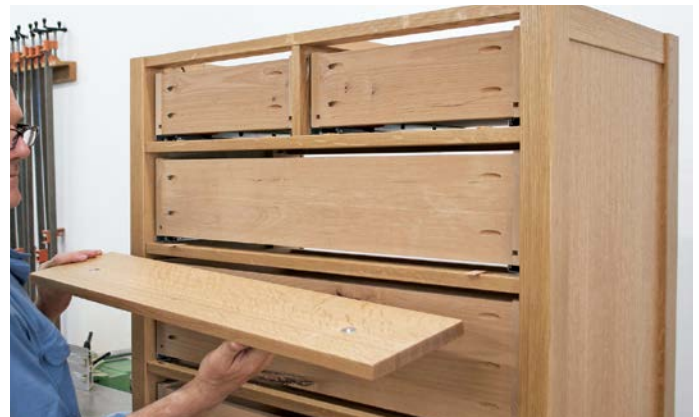
With shims in place on the drawer divider, set the drawer front into the opening and press to transfer the center mark.
