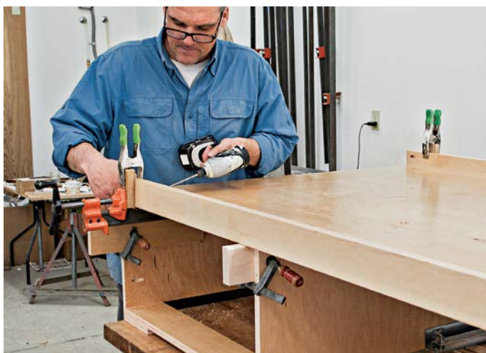
A bar clamp at the end and some small scraps of wood clamped to the partitions help support the back face frame as you attach it to the drawer cabinet.
