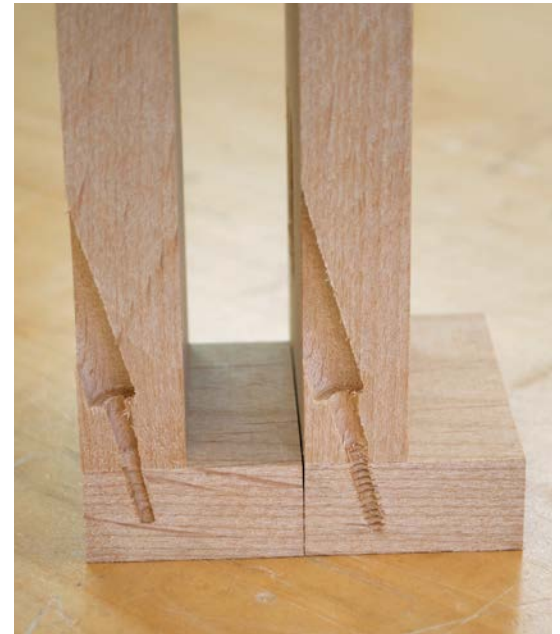
A deep \frac{3}{8} -in. predrill still leaves just enough material for the threads to bite.
