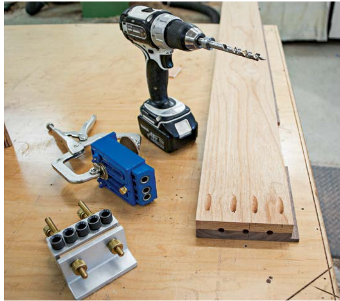
Dowels and pocket hole joinery work together to create strong, precise joints.
