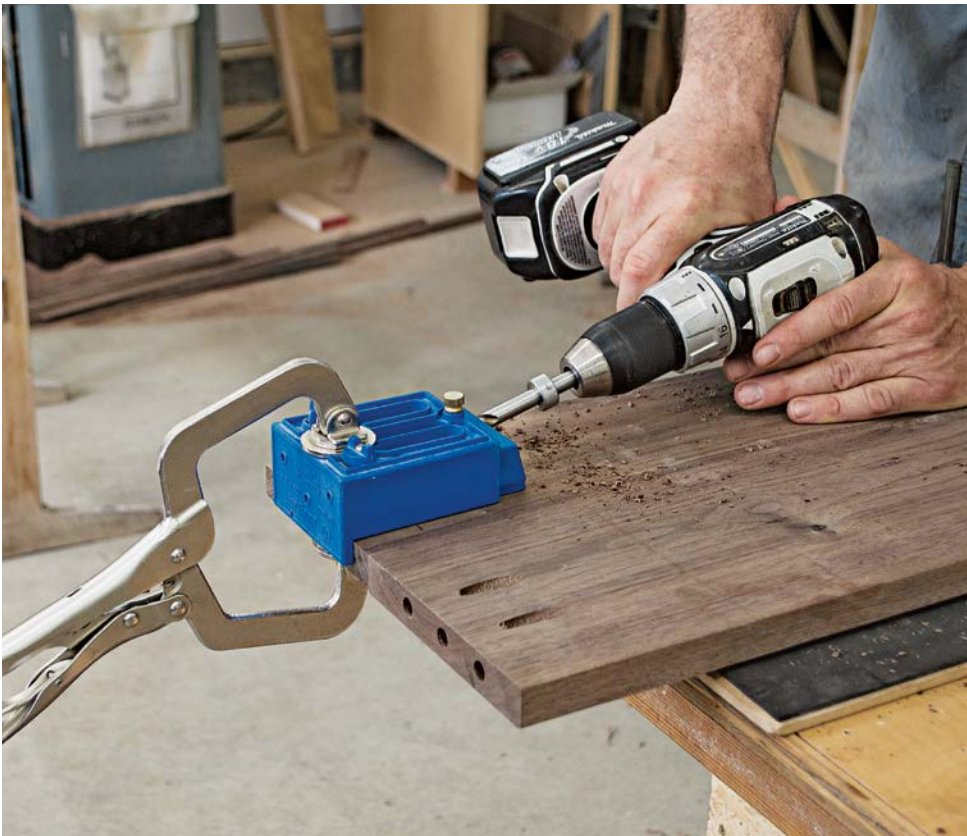
With the index pin set in the first pin of the doweling jig, drill for dowels in the third and fifth hole in the mattress rail.
