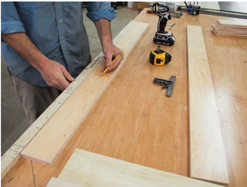
Use the story stick to help lay out the pocket holes in the front web-frame piece.
