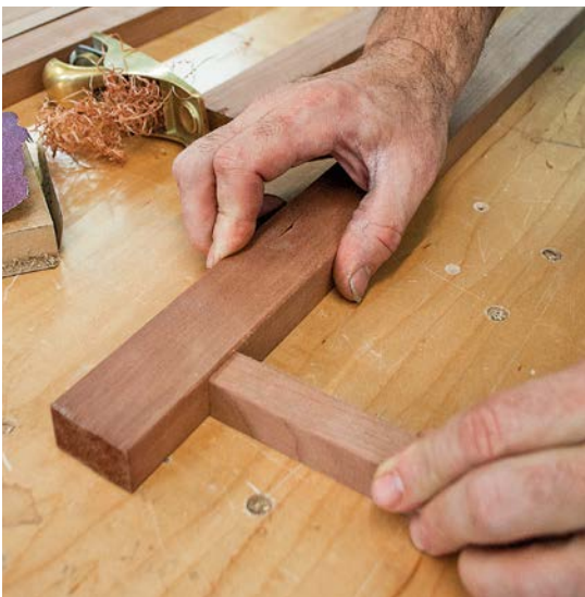
Check the roundover edges by butting a \frac{3}{4} -in. frame against the 1\frac{1}{2} -in. frame.
