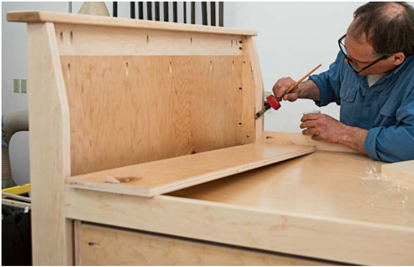
Apply glue to the biscuit holes in the furring strips and plywood panel.
