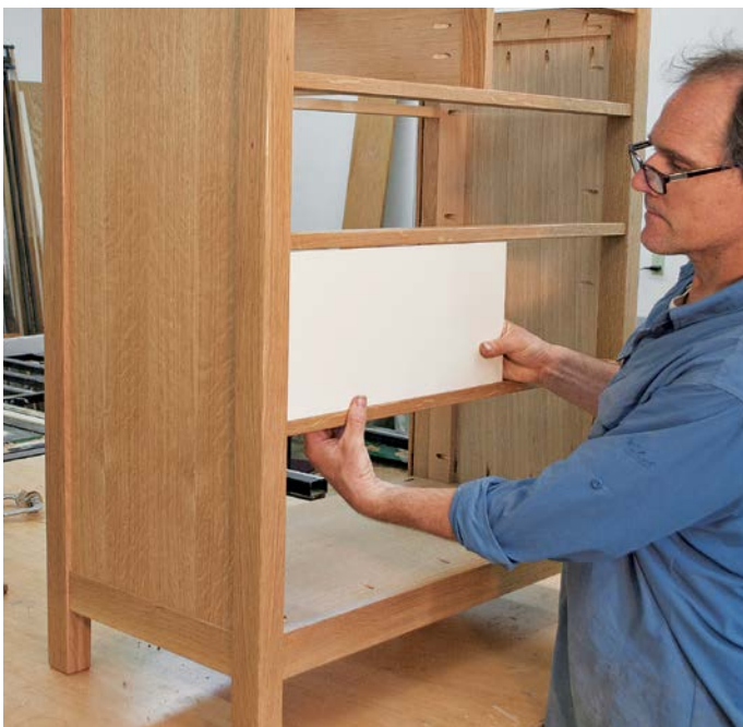
A scrap of MDF or other sheet material cut square at the end can help determine if the angle between the drawer divider and the post is square.
