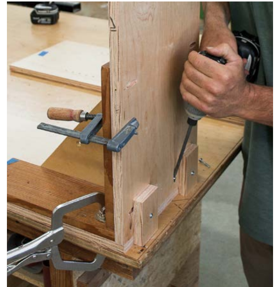
You can use the right-angle jig and small blocks of wood instead of a bar clamp to secure the side to the bottom while pocket screwing.
