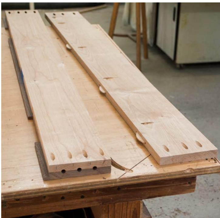
Cut biscuits in the bottom headboard rail and the alder rail. Pocket holes, biscuits, and dowels work together to ensure an accurate fit.
