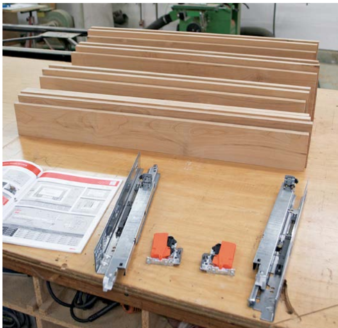
Rip the drawer parts to width, then separate into drawer groups. Shown at front are the Tandem drawer slides with locking clips (and spec sheet).
