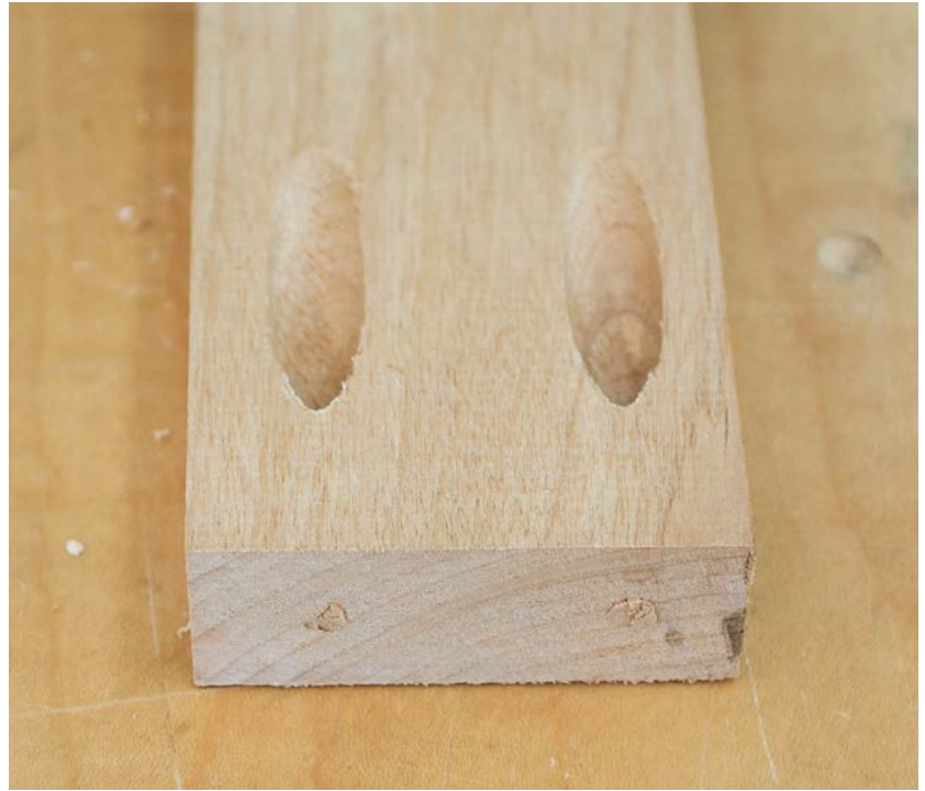
End-grain popout occurs when a little piece of wood at the tip of a predrilled hole comes unseated.
