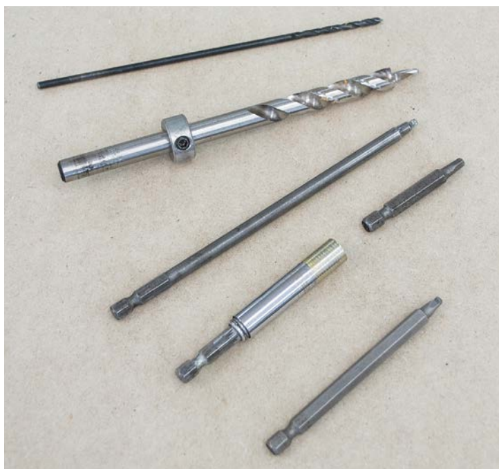
Drill bits and drivers, from the top: a 1/8-in. extra-long predrill bit; a 3/8-in. stepped pocket hole drill bit; a 6-in. square driver; a 2-in. square driver and extension; and a 3-in. square driver.
