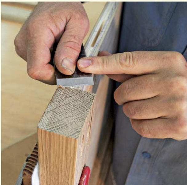
Using a sharp plane blade or chisel, pare the end grain of the rail so that it is flush with the panel side.
