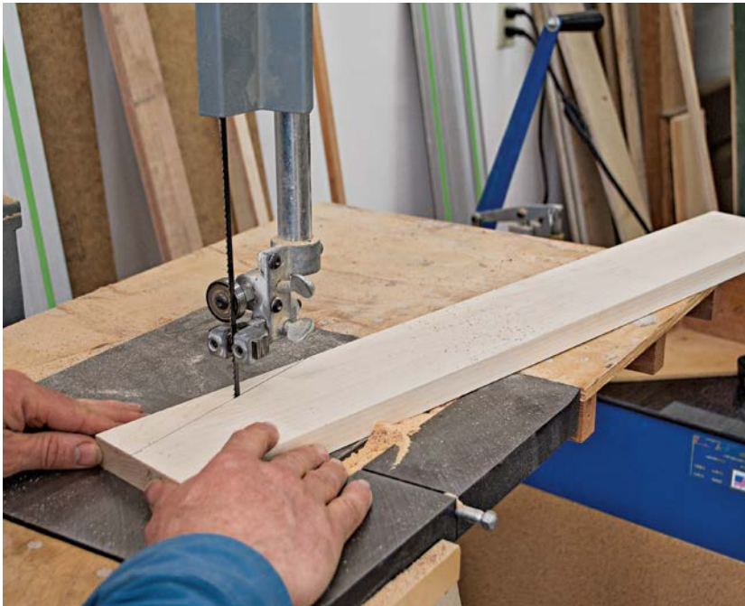
Add a bit of flair to the corner posts by cutting a taper.
