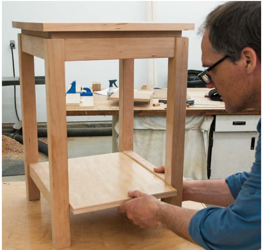
Slide the test shelf into place, making sure that the fit is not too tight and the shadow line between the shelf and the stretchers is consistent.
