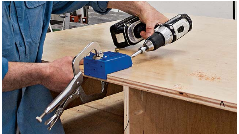
The portable pocket screw jig is handy for very large panels that would be difficult to drill in the benchtop jig.
