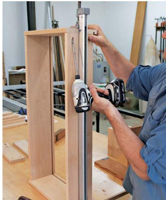
Clamp across the drawer width when driving pocket screws into the drawer sides.
