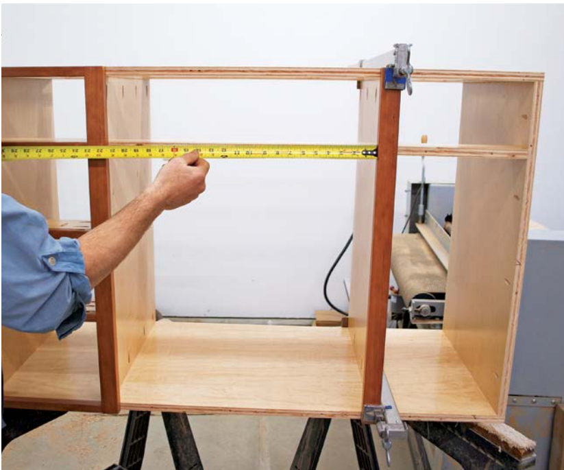
Clamp the third vertical frame piece so that the drawer-side edge is flush with the plywood partition and then measure the sink opening.
