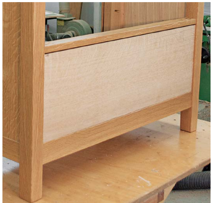
Cut and sand the drawer fronts until there is an even \frac{1}{16} -in. reveal on all four sides.
