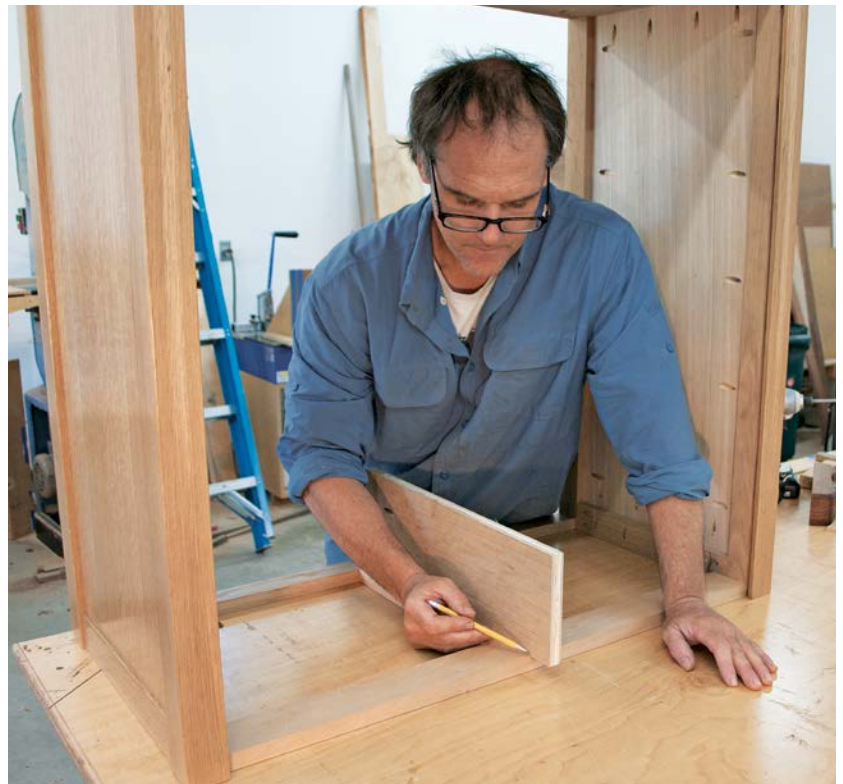
Place the top drawer partition in position and mark its length.
