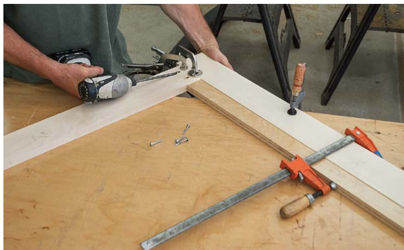
Clamp the top spacer to the top rail to locate the stiles exactly \frac{1}{16} in. less than the cabinet opening, then attach the stile to the top rail with two pocket screws.
