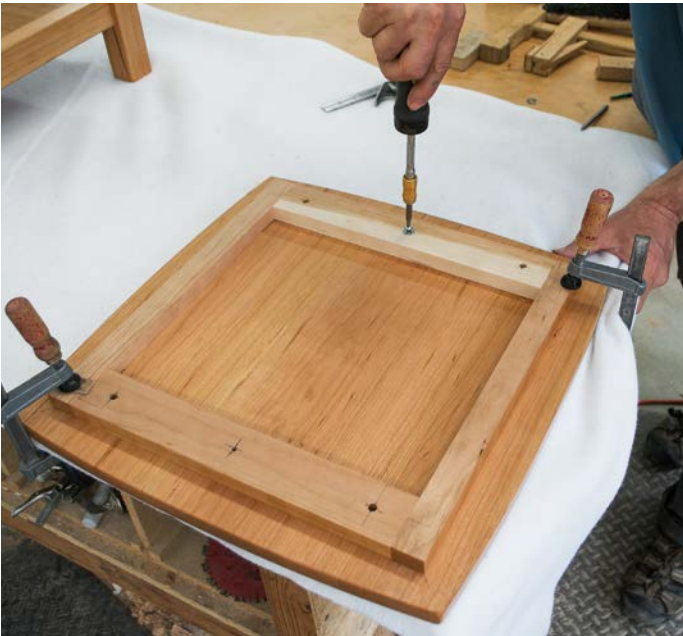
Attach the spacer frame to the tabletop with pocket screws and #10 washers, driving the screws by hand.
