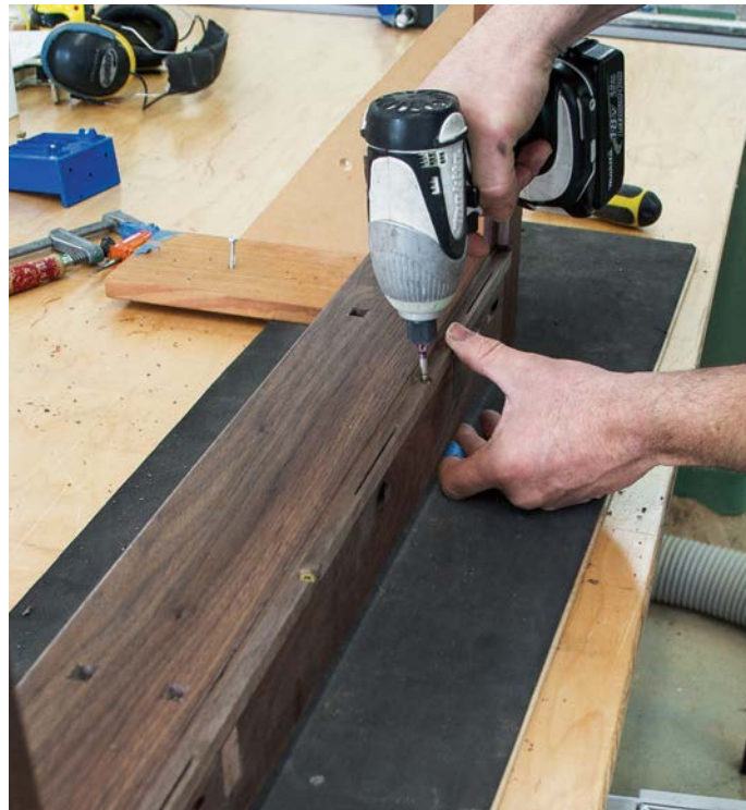
An additional screw through the rabbet of the shelf into the bottom rail helps close up any gaps between the two and adds some strength.
