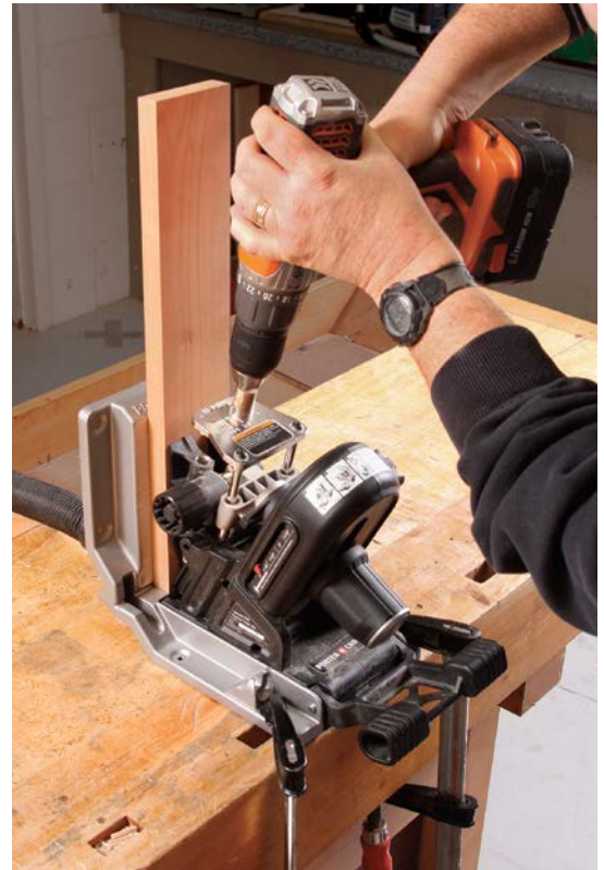
Drilling goes quickly with the Porter-Cable QuikJig, and a handy scale on the side tells you the screw length you need for your setup.
