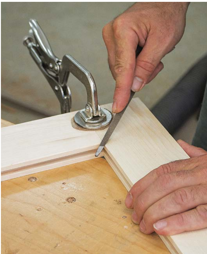
Chamfer the inside corner of the back frame panel with a tri-angle file before assembly (the spot is hard to reach once the frame and panel are assembled).
