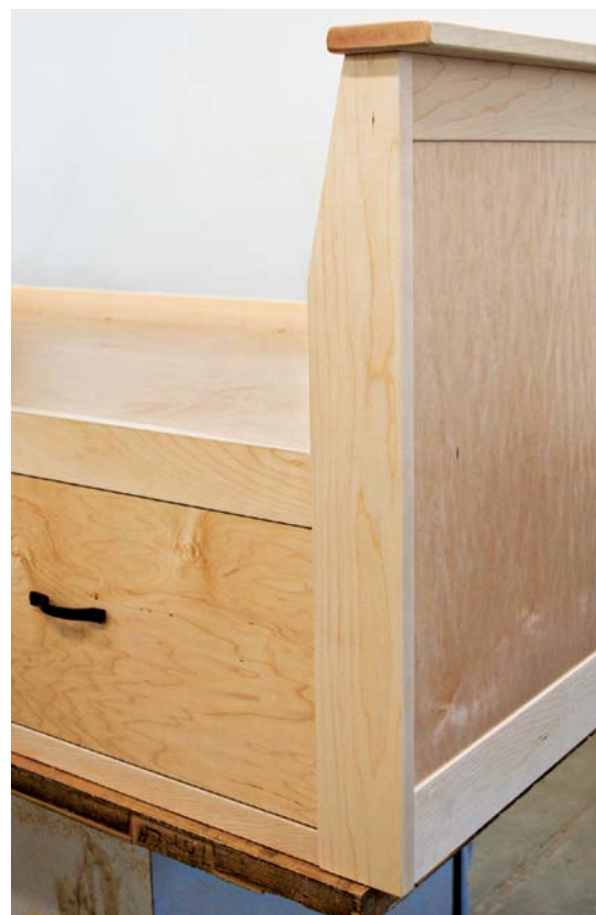
With pocket hole joinery, you can create strong joints without a single screw or screw hole visible. This is a detail of the daybed project (see p. 77).
