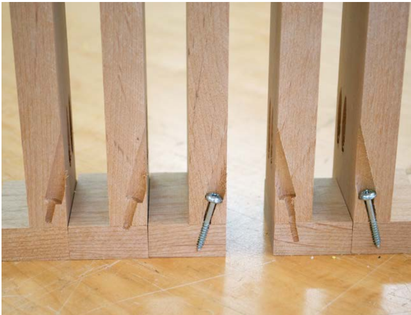
The pocket holes on the left were predrilled \frac{1}{8} in. deep to minimize shift. The pocket holes on the right were predrilled \frac{3}{8} in. deep to minimize stress.
