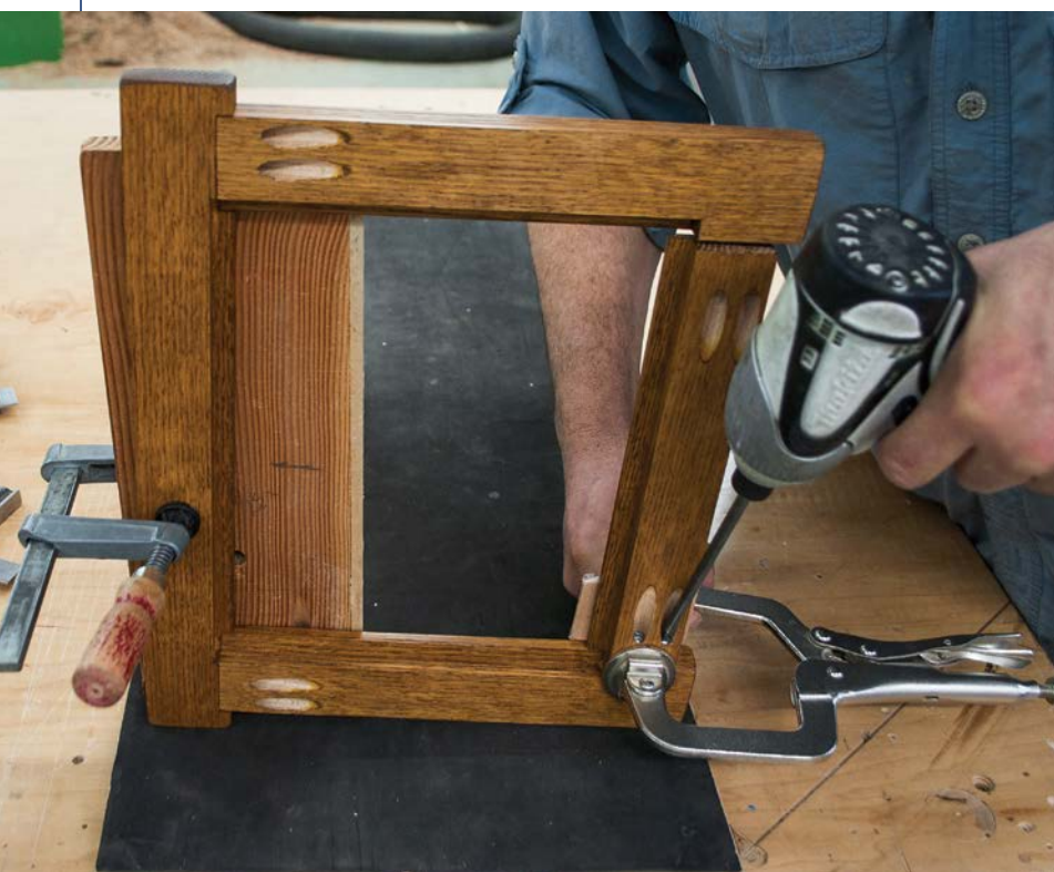
Use the right-angle jig to hold the top rail of the picture frame while driving the pocket screws from the stile.
