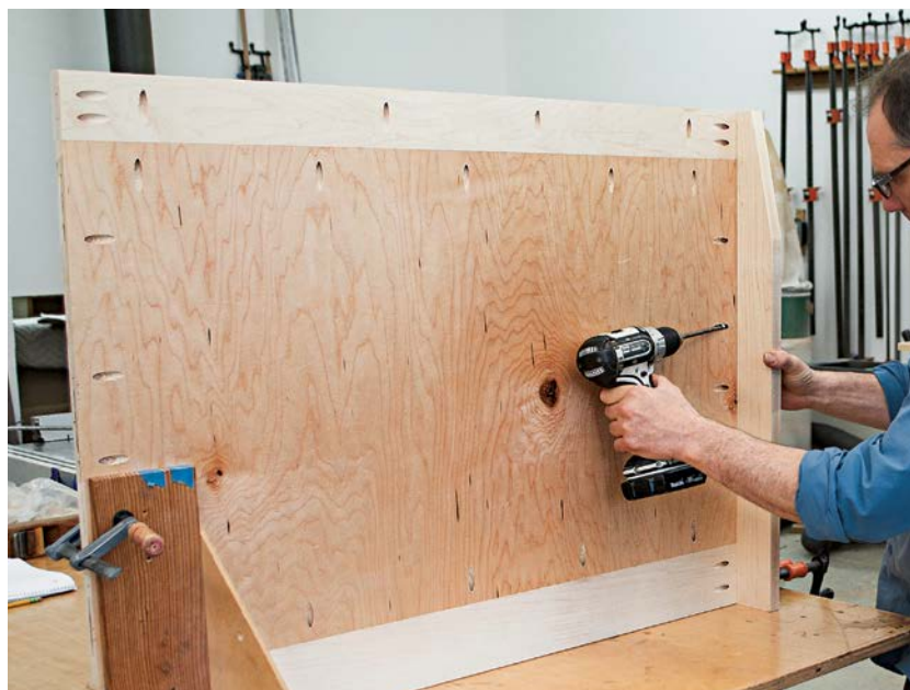
Biscuits keep the joint from shifting so it's not necessary to use clamps in addition.
