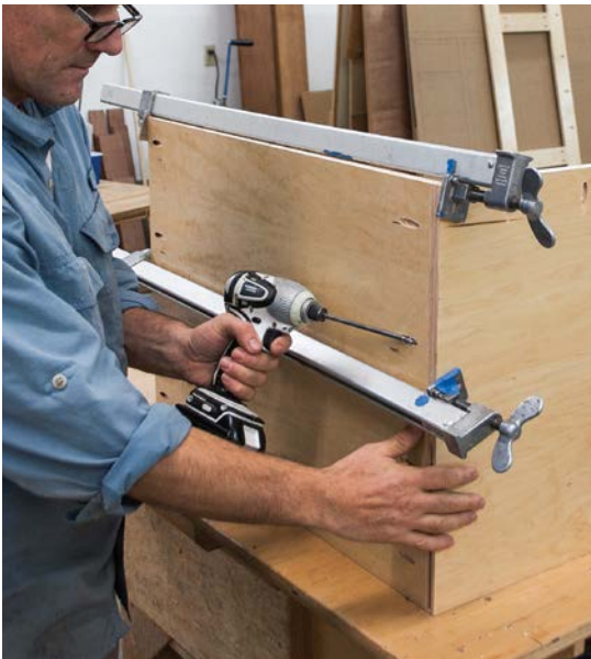
Clamps at each screw hole help ensure that the parts do not shift during assembly.
