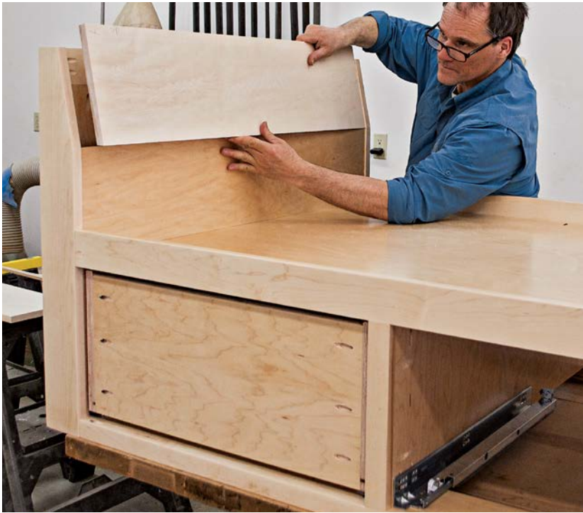
Slide the upper panel into place to test the fit of the bevel cut.
