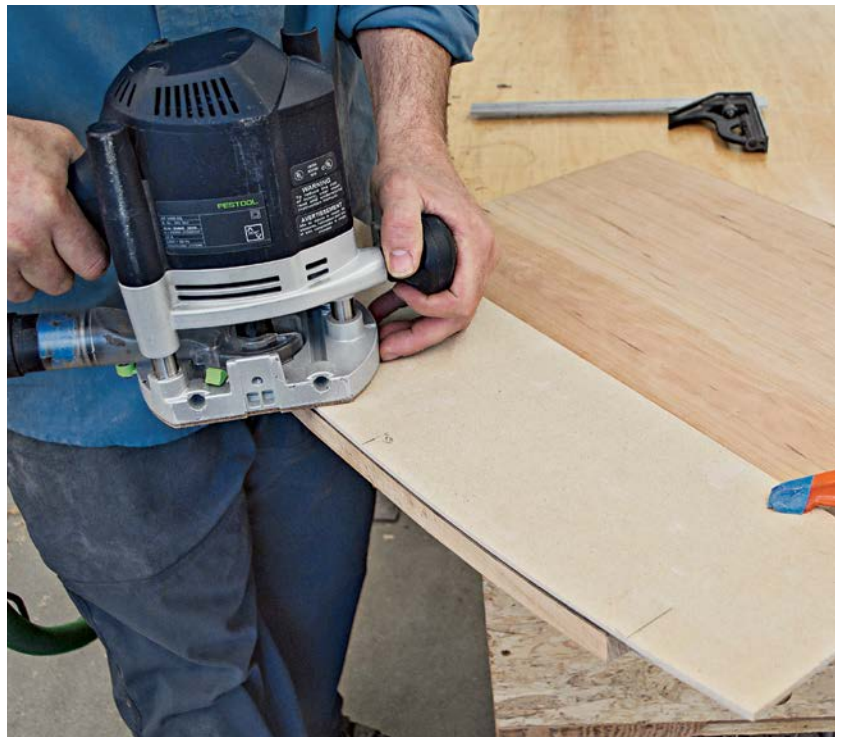
Use a router with a bearing in the middle to follow the template and clean up the sawmarks.
