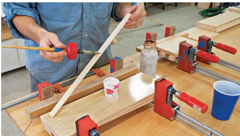
Apply glue to the edge-band. (Note the three clamping stations.)
