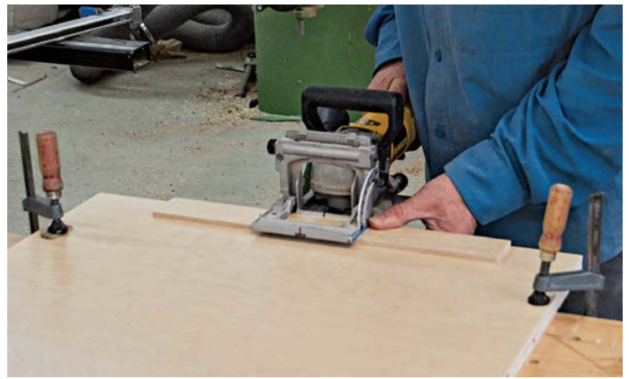
Use a 1/4-in. shim with the biscuit joiner to create the step between the corner post and the end panel.
