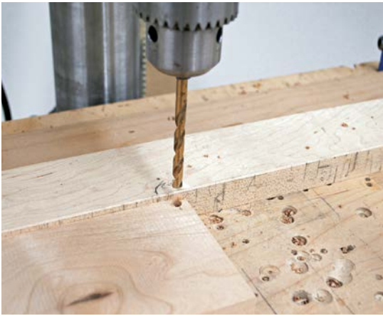
Use a drill press and fence to drill the index holes in the drawer backs.
