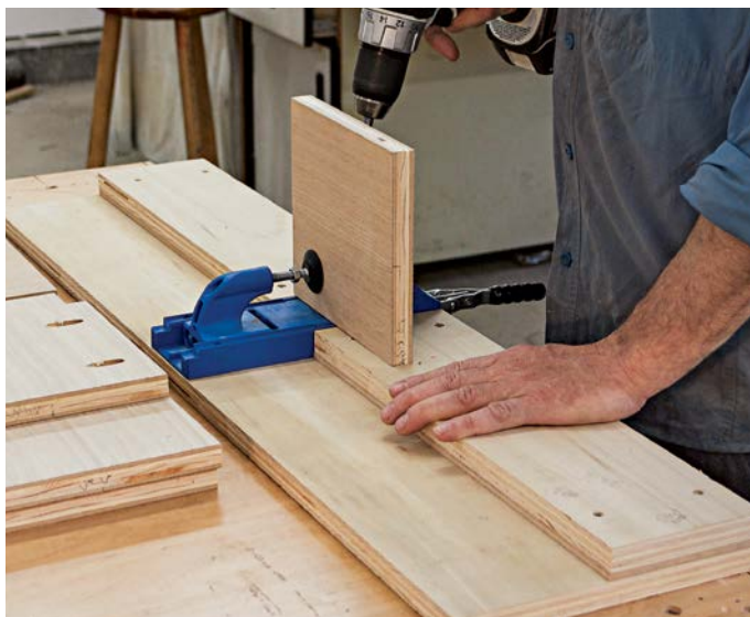
Use the benchtop jig to drill holes in the plywood panels.
