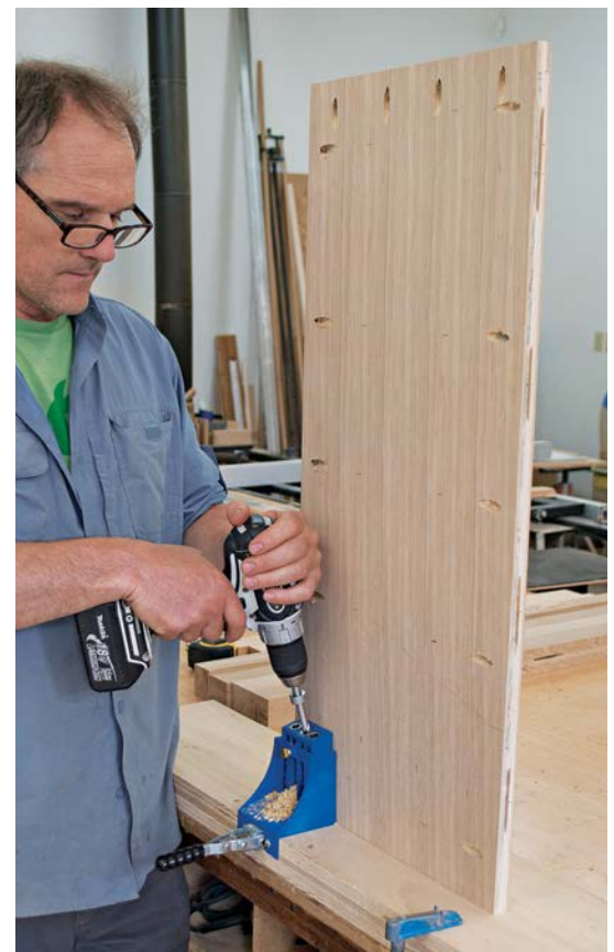
Drill pocket holes in the panels to attach the rails and posts.
