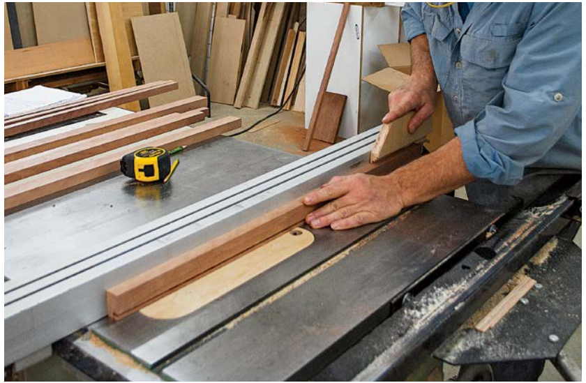
Cut a rabbet in the back edge of the vertical frame member that butts against the wall so that it is easier to scribe during installation.
