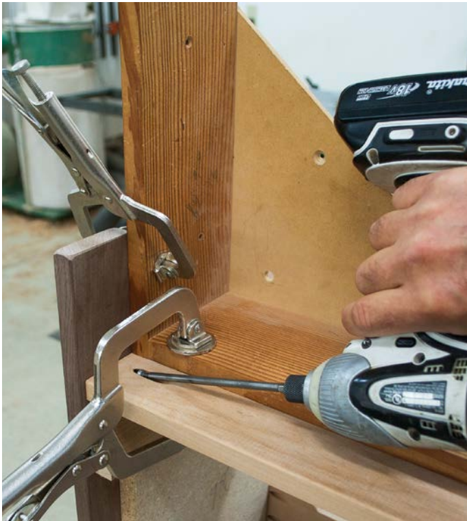
Clamp the right-angle jig to the shelf and bench end so that the first pocket hole is uncovered.
