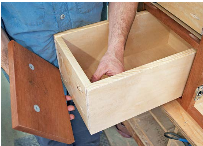
Thread the #8-32 screws into the plastic plug locaters in the drawer front (left), then add two pocket screws to secure the drawer front in its final location (above).
