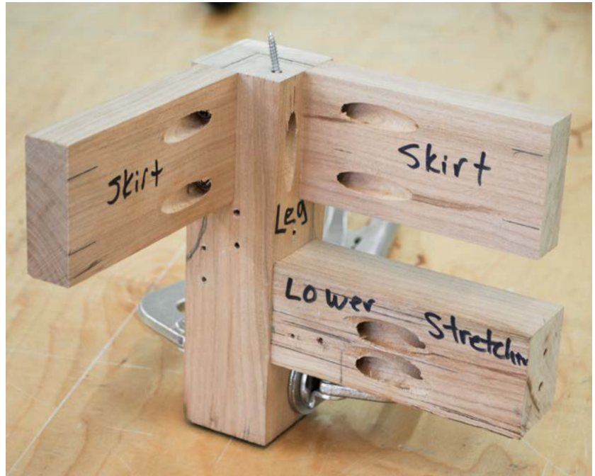
The author uses offcuts to mock up the pocket screw locations at the corners and where the lower stretcher meets the legs.
