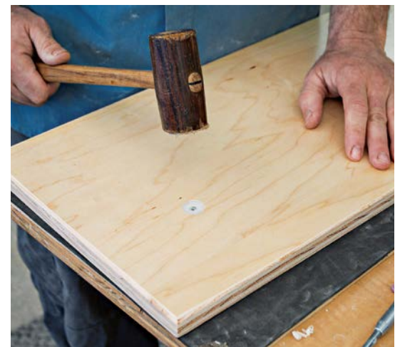
Installing drawer front locaters into the back of the drawer fronts makes it easy to achieve an even reveal on all four sides.
