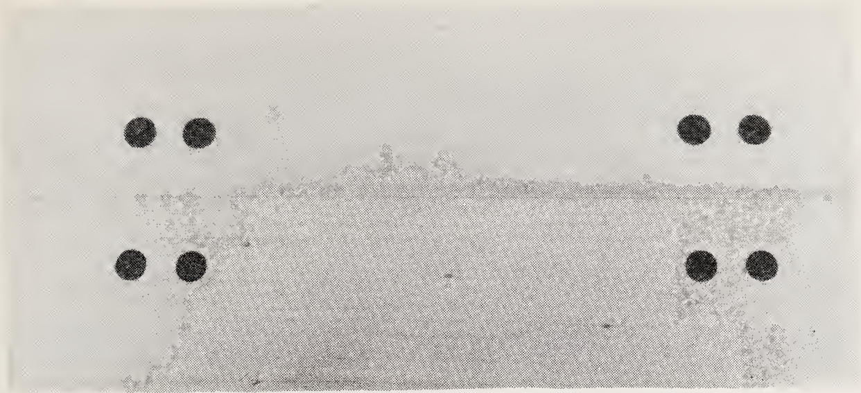
Figure 38 Contrasting dowels used in the edge joint.
