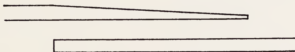
Diagram 252 The opposite end of the strip of timber should be tapered to prevent thickness at the joint.
