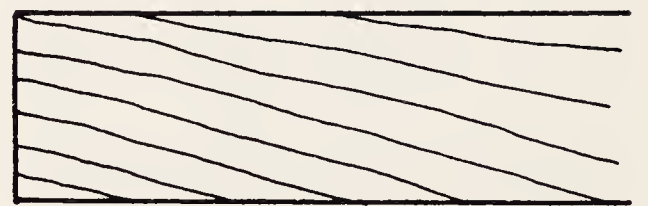
Diagram 1 Planing should follow the same direction as the grain to prevent the tearing of timber fibres
