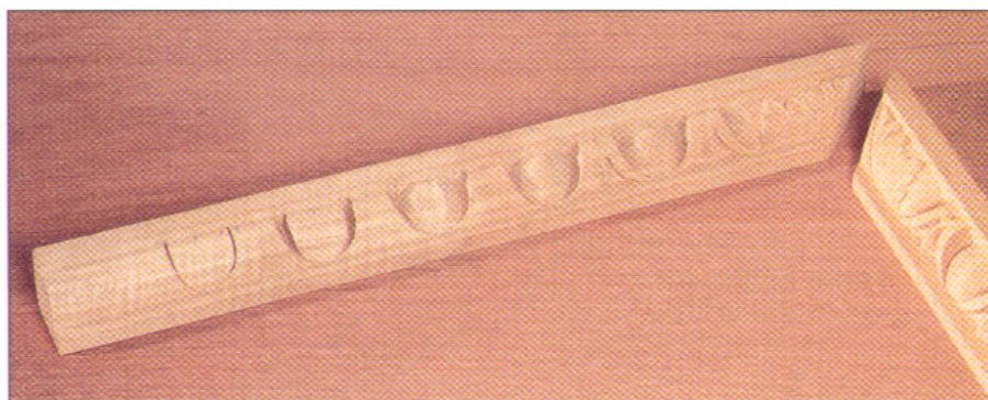
The egg-and-dart pattern shown above was carved in ovolo-shaped molding. The piece on the right is finished; the sample piece on the left shows the progression of required steps. Acanthus motifs at the corner will allow the mitered ends to butt together cleanly.
