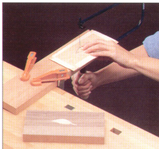
A fret saw is used with a bird's-mouth table to cut veneer for marquetry. The table features a V-cutout to accommodate the saw. For the cut shown above, the table is shimmed to create a bevel on the cut edges, ensuring seamless joints between the pieces of veneer.
