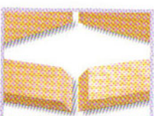
Compound miter by machine page 126
