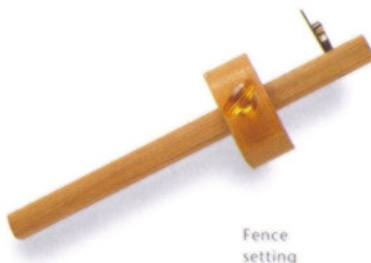
Scribing knife makes finest line.
