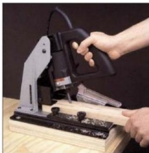
The commercial jig shown above cuts accurate pocket holes with a minimum of setup time. With the workpiece clamped in the jig, the router-like cutter is pivoted into the face of the board to cut the pocket hole.
