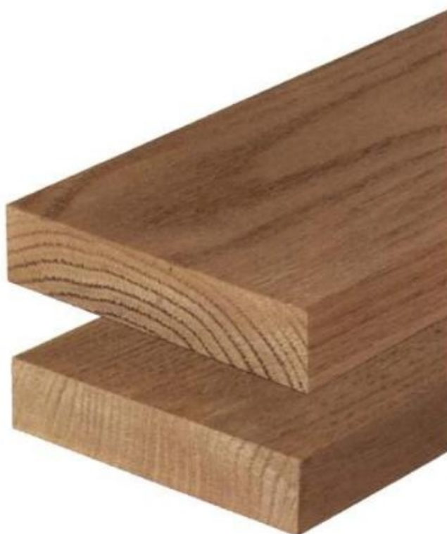
The annual growth rings in the plain-sawn oak board ( top ) appear on the face as an elliptical landscape figure. Plain-sawn stock is sliced tangent to the rings. The growth rings in the quartersawn oak board ( bottom ) appear as lines perpendicular to the face.
