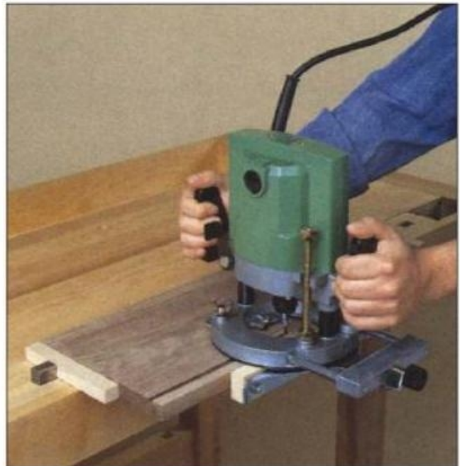
A straight bit carves a groove in a board. Riding an edge guide along the board produces a cut parallel to the edge.
