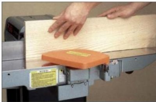
A jointer produces a smooth, straight, even edge. Gluing jointed boards together edge-to-edge will form a panel that is every bit as strong as a single piece of lumber.
