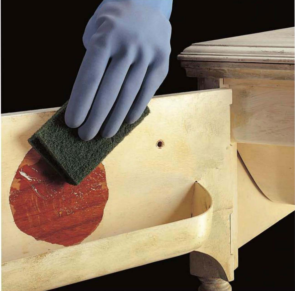
Partially strip finish in an inconspicuous area so you can examine the wood more closely (strip a large enough section to allow you to evaluate how effectively the chemical stripper dissolves the paint, too).
