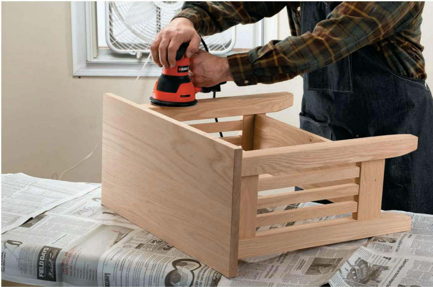
Sand wood with power sanders , like the random-orbit sander shown above, to make quick work of the initial finish sanding stages, while producing a very smooth wood surface.
