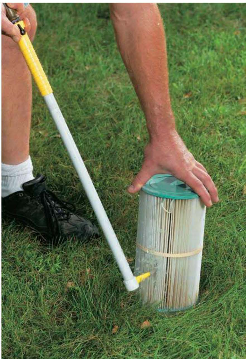
A filter-cleaning nozzle directs water from a hose into the filter pleats for a more thorough cleaning that will not damage the filter material.
