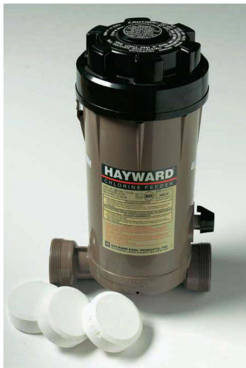
An inline chlorinator for a swimming pool, sometimes called a mechanical feeder, dispenses measured amounts of sanitizing chemicals at a constant rate.
